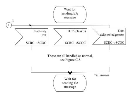
Figure C.9/Q.714 – Expedited data transfer procedures at relay node with coupling for SCCP connection-oriented control (SCOC) (sheet 2 of 2)
