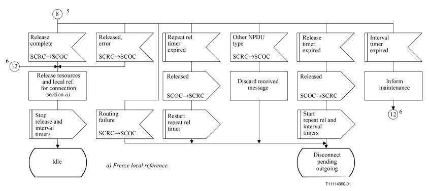
Figure C.7/Q.714 – Connection release procedures at relay node with coupling for SCCP connection-oriented control (SCOC) (sheet 6 of 9)
