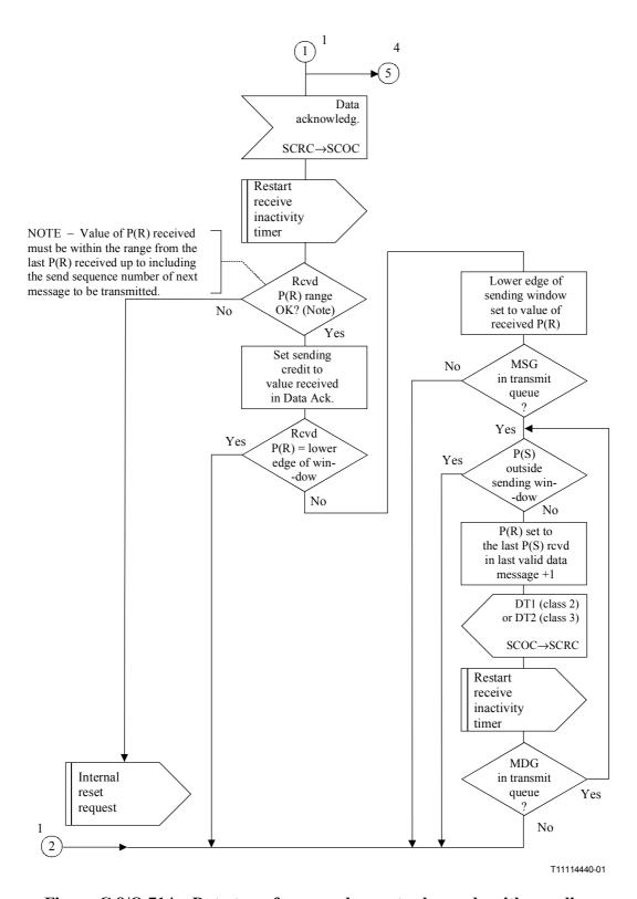
Figure C.8/Q.714 – Data transfer procedures at relay node with coupling for SCCP connection-oriented control (SCOC) (sheet 2 of 4)
