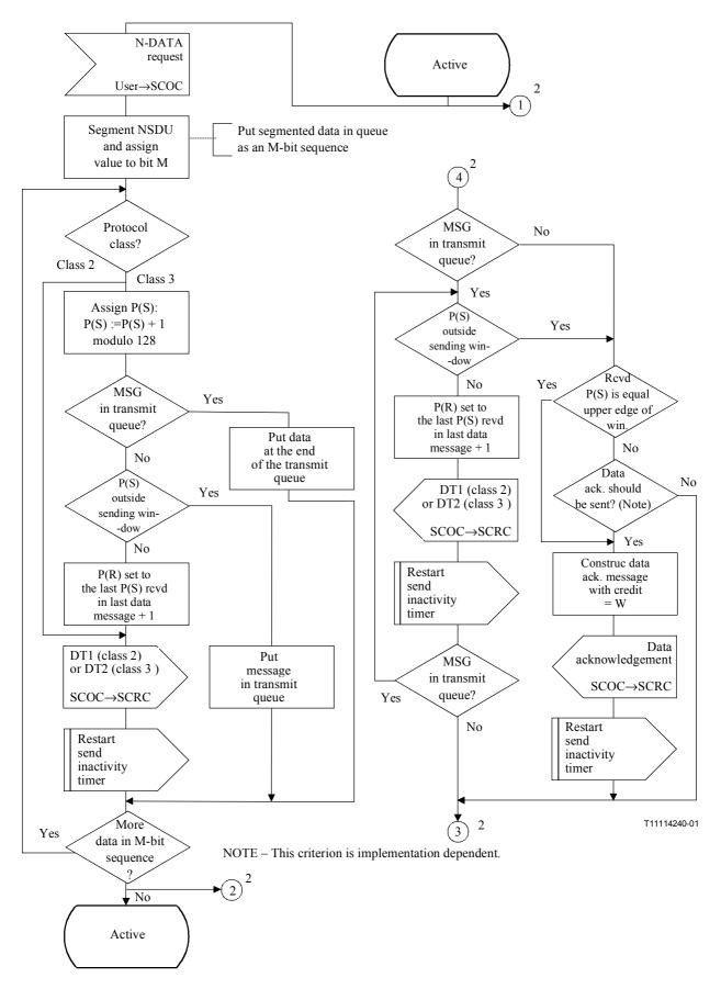
Figure C.4/Q.714 – Data transfer procedures at originating and destination nodes for SCCP connection-oriented control (SCOC) (sheet 1 of 4)
