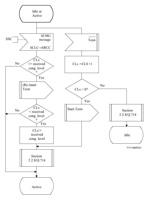
Figure D.13/Q.714 – Remote SCCP and nodal congestion control (SRCC) (sheet 1 of 2)
