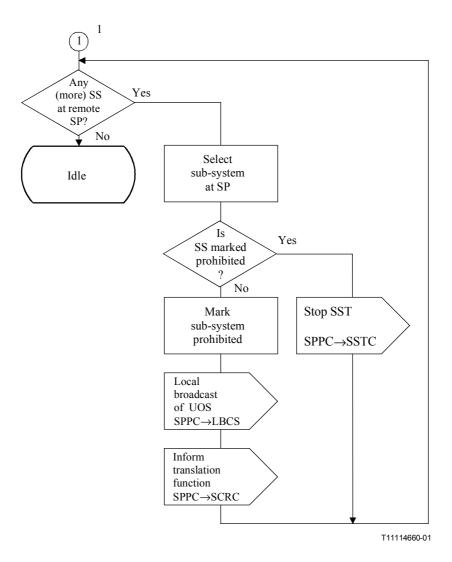
Figure D.2/Q.714 – Signalling point prohibited control (SPPC) (sheet 2 of 2)
