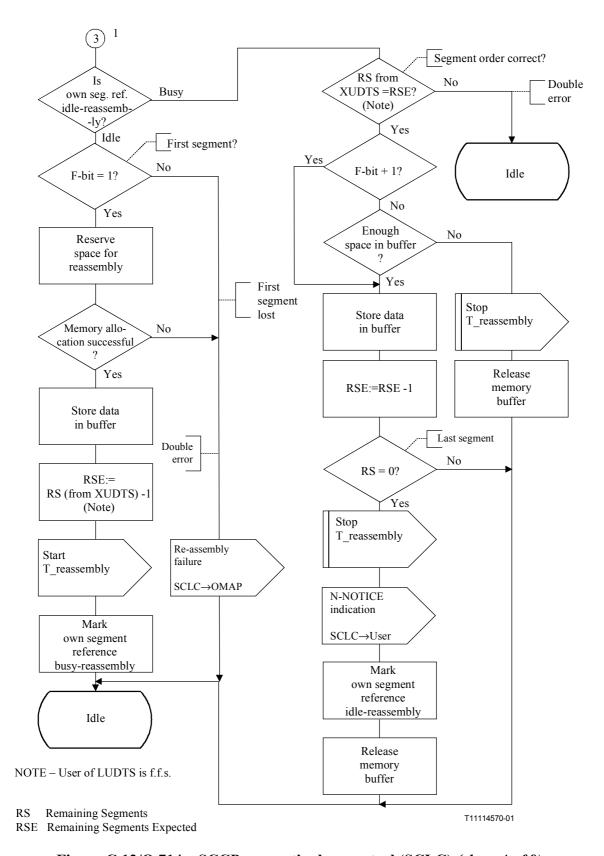
Figure C.12/Q.714 – SCCP connectionless control (SCLC) (sheet 4 of 9)
