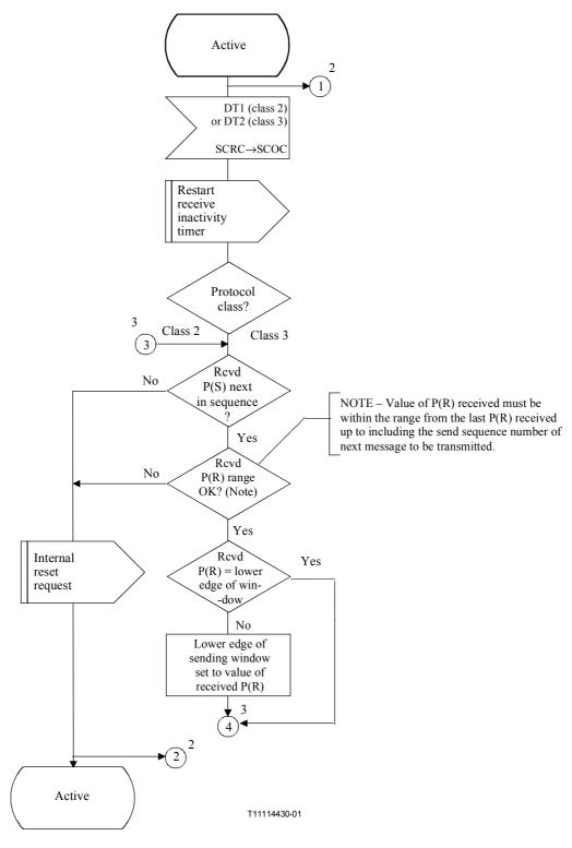
Figure C.8/Q.714 – Data transfer procedures at relay node with coupling for SCCP connection-oriented control (SCOC) (sheet 1 of 4)
