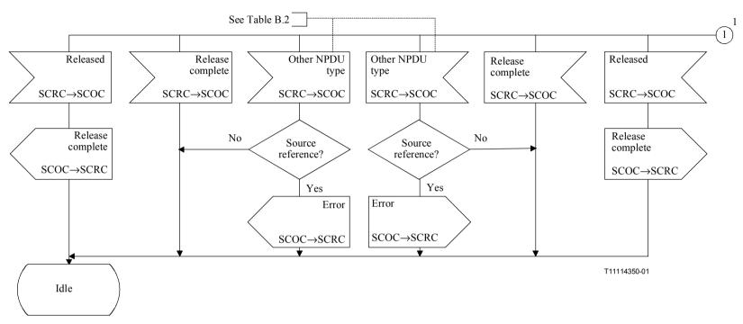
Figure C.7/Q.714 – Connection establishment procedures at relay node with coupling for SCCP connection-oriented control (SCOC) (sheet 2 of 9)
