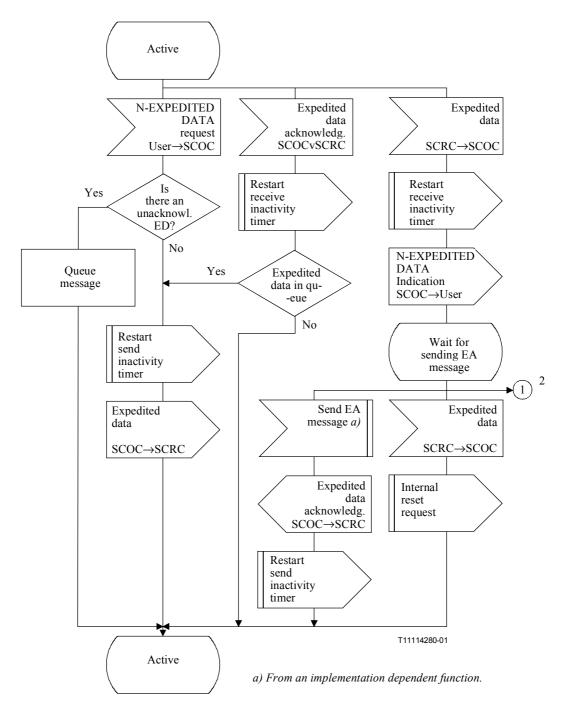
Figure C.5/Q.714 – Expedited data transfer procedures at originating and destination nodes for SCCP connection-oriented control (SCOC) (sheet 1 of 2)
