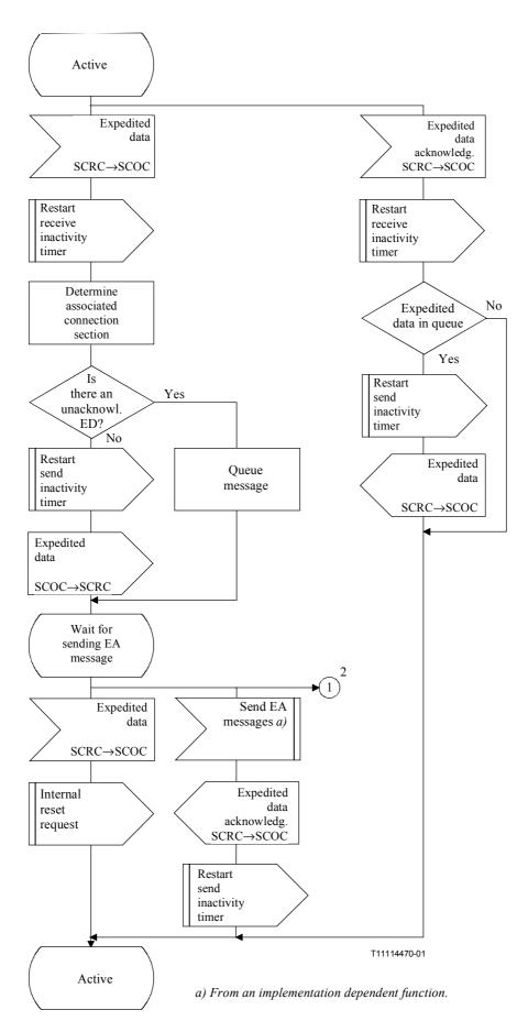
Figure C.9/Q.714 – Expedited data transfer procedures at relay node with coupling for SCCP connection-oriented control (SCOC) (sheet 1 of 2)
