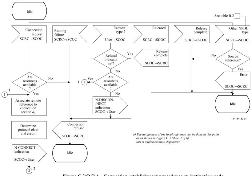
Figure C.3/Q.714 – Connection establishment procedures at destination node for SCCP connection-oriented control (SCOC) (sheet 1 of 6)
