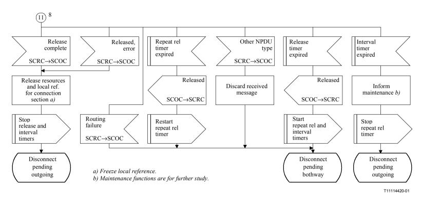
Figure C.7/Q.714 – Connection release procedures at relay node with coupling for SCCP connection-oriented control (SCOC) (sheet 9 of 9)
