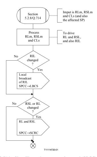
Figure D.4/Q.714 – Signalling point congested control (SPCC) (sheet 4 of 4)
