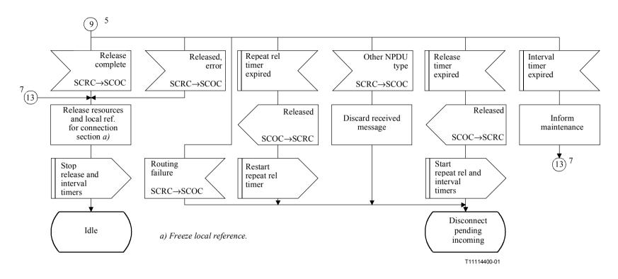
Figure C.7/Q.714 – Connection release procedures at relay node with coupling for SCCP connection-oriented control (SCOC) (sheet 7 of 9)
