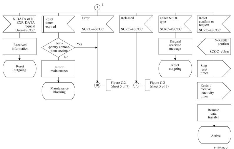
Figure C.6/Q.714 – Reset procedures at originating and destination nodes for SCCP connection-oriented control (SCOC) (sheet 2 of 4)
