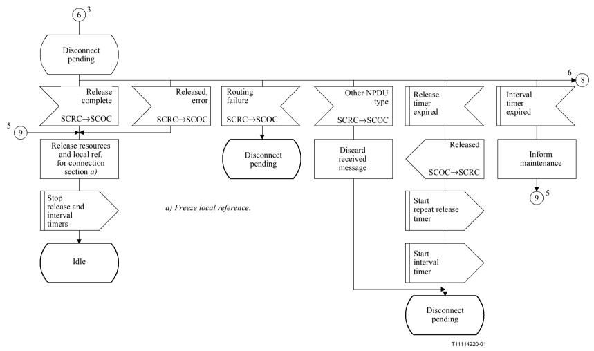
Figure C.3/Q.714 – Connection release procedures at destination node for SCCP connection-oriented control (SCOC) (sheet 5 of 6)
