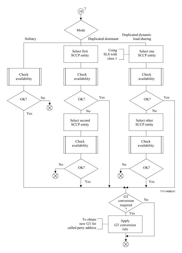
Figure C.1/Q.714 – SCCP routing control procedures (SCRC) (sheet 8 of 12)
