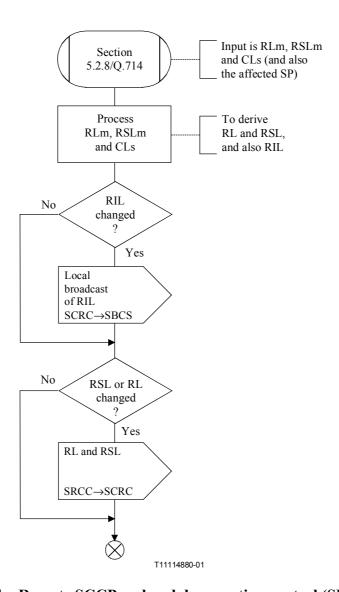
Figure D.13/Q.714 – Remote SCCP and nodal congestion control (SRCC) (sheet 2 of 2)
