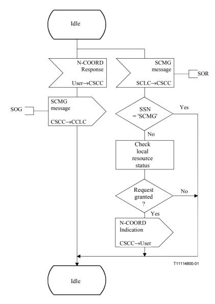
Figure D.8/Q.714 – Coordinated state change control (CSCC) at the requesting node (sheet 2 of 2)
