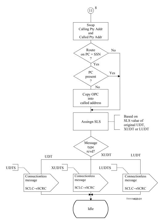
Figure C.12/Q.714 – SCCP connectionless control (SCLC) (sheet 9 of 9)
