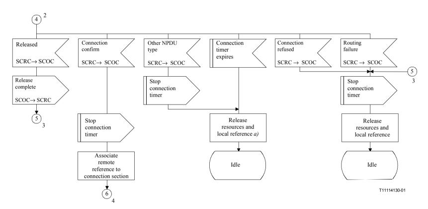
Figure C.2/Q.714 – Connection establishment procedures at originating node for SCCP connection-oriented control (SCOC) (sheet 3 of 7)
