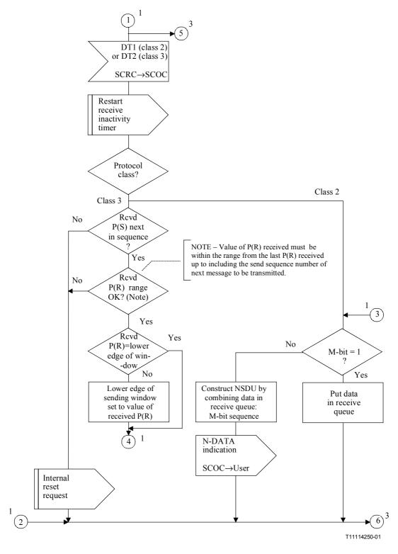
Figure C.4/Q.714 – Data transfer procedures at originating and destination nodes for SCCP connection-oriented control (SCOC) (sheet 2 of 4)
