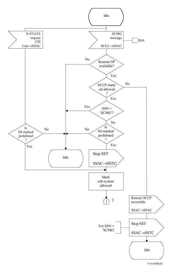
Figure D.6/Q.714 – Subsystem allowed control (SSAC) (sheet 1 of 2)
