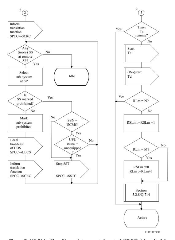
Figure D.4/Q.714 – Signalling point congested control (SPCC) (sheet 3 of 4)
