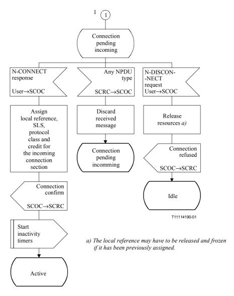
Figure C.3/Q.714 – Connection establishment procedures at destination node for SCCP connection-oriented control (SCOC) (sheet 2 of 6)
