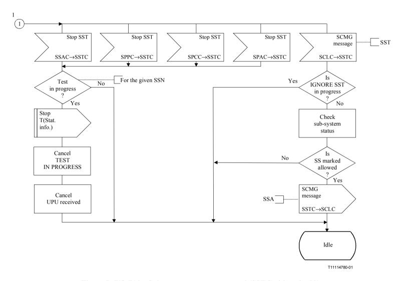
Figure D.7/Q.714 – Subsystem status test control (SSTC) (sheet 2 of 2)
