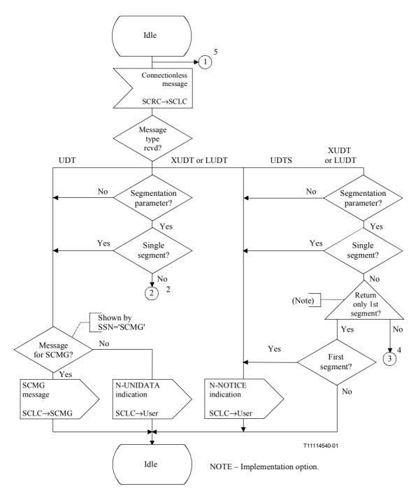
Figure C.12/Q.714 – SCCP connectionless control (SCLC) (sheet 1 of 9)
