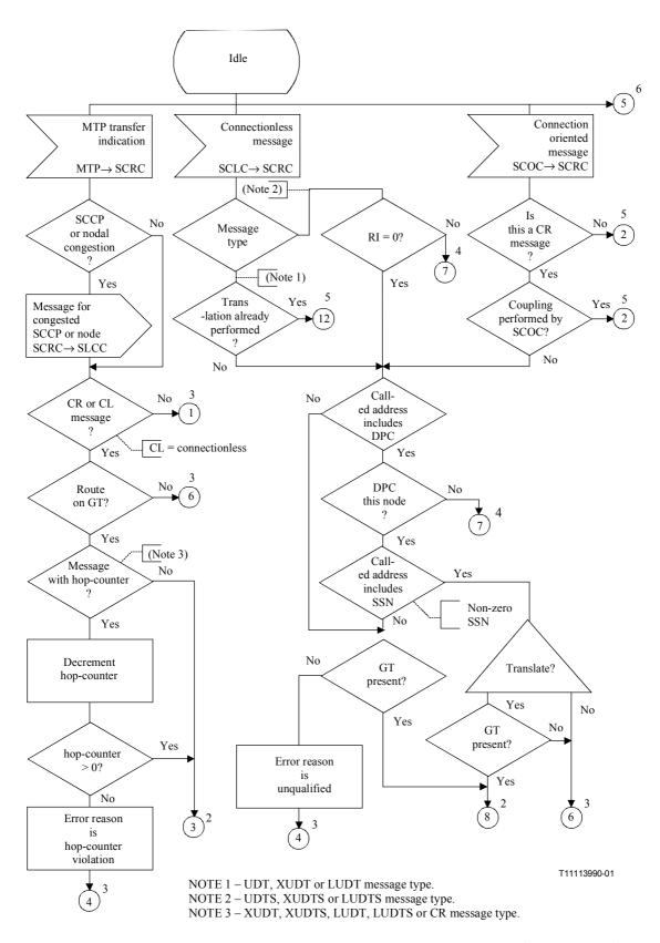
Figure C.1/Q.714 – SCCP routing control procedures (SCRC) (sheet 1 of 12)
