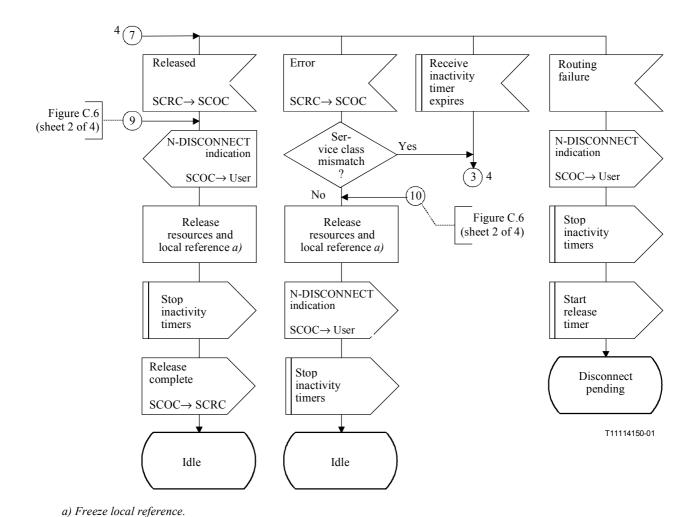
Figure C.2/Q.714 – Connection release procedures at originating node for SCCP connection-oriented control (SCOC) (sheet 5 of 7)
