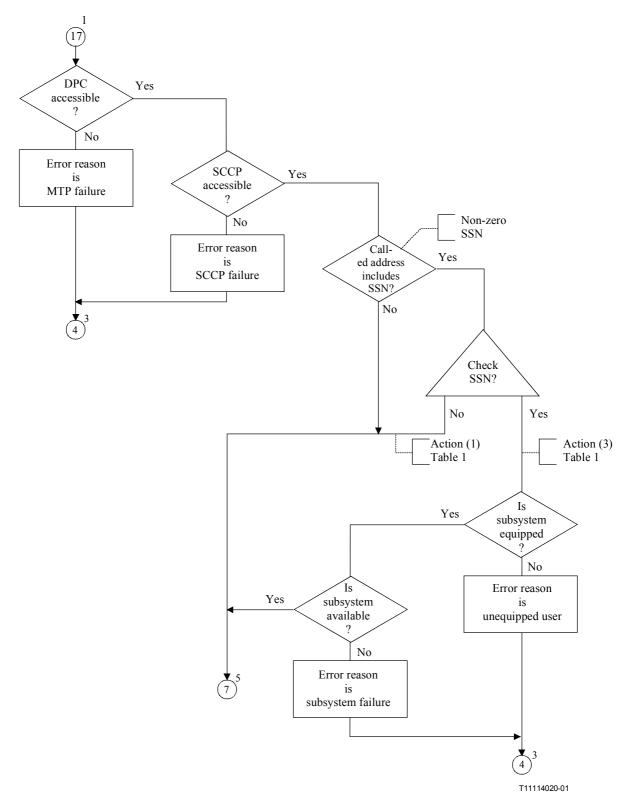
Figure C.1/Q.714 – SCCP routing control procedures (SCRC) (sheet 4 of 12)
