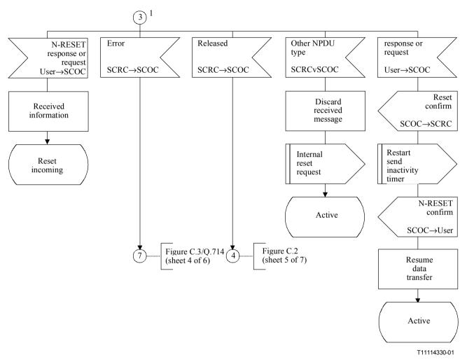
Figure C.6/Q.714 – Reset procedures at originating and destination nodes for SCCP connection-oriented control (SCOC) (sheet 4 of 4)
