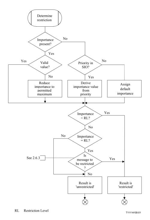
Figure C.1/Q.714 – SCCP routing control procedures (SCRC) (sheet 12 of 12)
