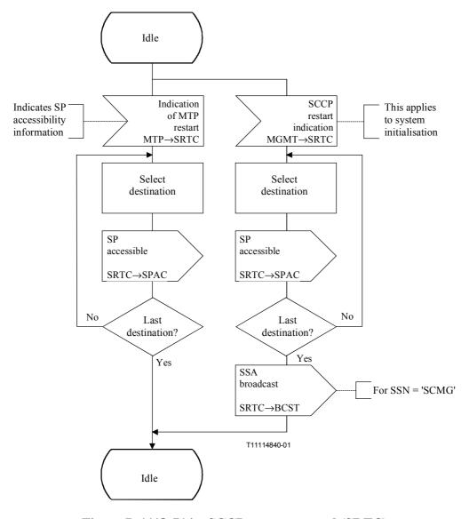
Figure D.11/Q.714 – SCCP restart control (SRTC)
