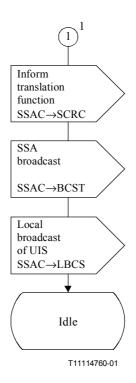
Figure D.6/Q.714 – Subsystem allowed control (SSAC) (sheet 2 of 2)
