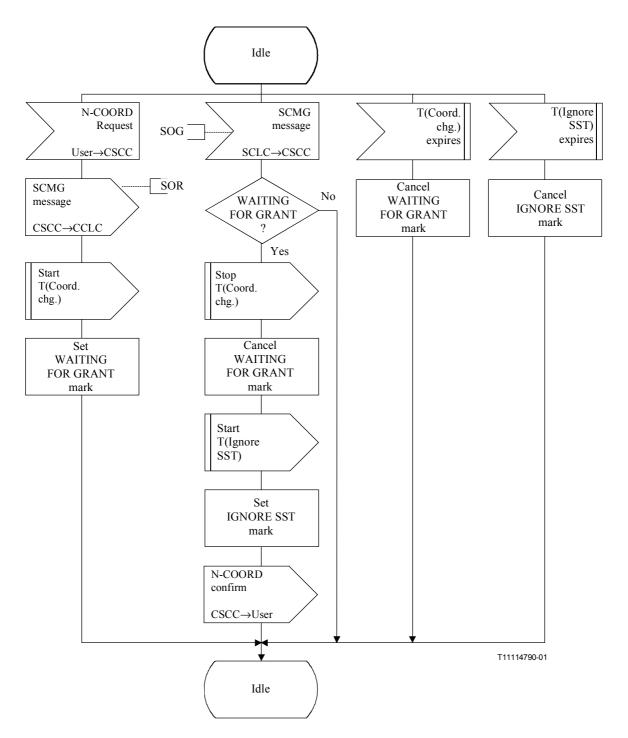
Figure D.8/Q.714 – Coordinated state change control (CSCC) at the requesting node (sheet 1 of 2)
