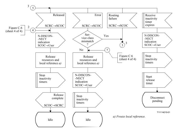
Figure C.3/Q.714 – Connection release procedures at destination node for SCCP connection-oriented control (SCOC) (sheet 4 of 6)
