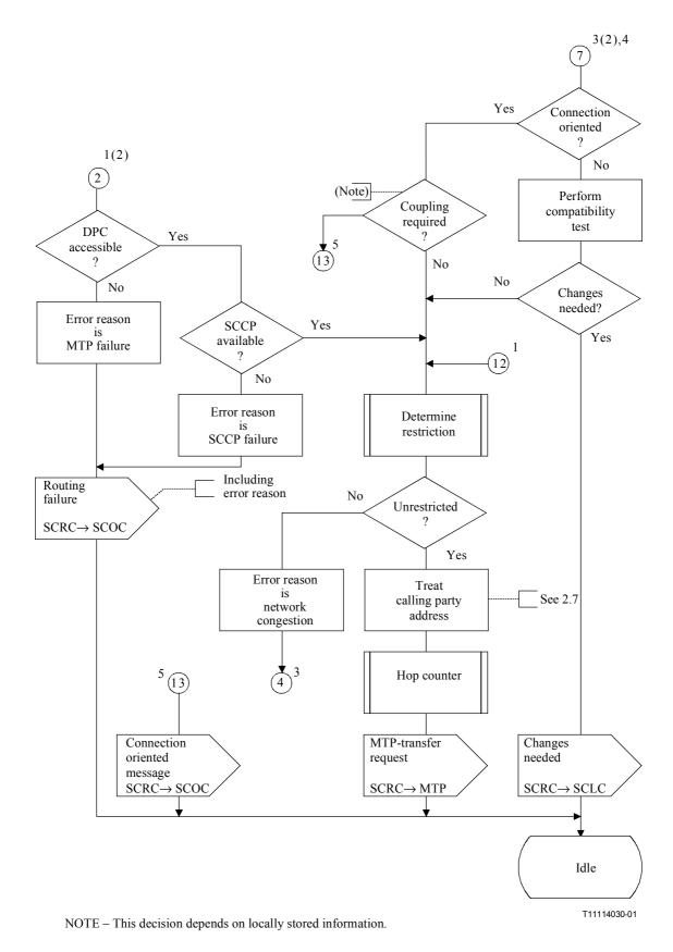
Figure C.1/Q.714 – SCCP routing control procedures (SCRC) (sheet 5 of 12)
