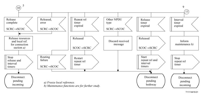
Figure C.7/Q.714 – Connection release procedures at relay node with coupling for SCCP connection-oriented control (SCOC) (sheet 8 of 9)
