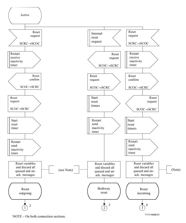
Figure C.10/Q.714 – Reset procedures at relay node with coupling for SCCP connection-oriented control (SCOC) (sheet 1 of 4)
