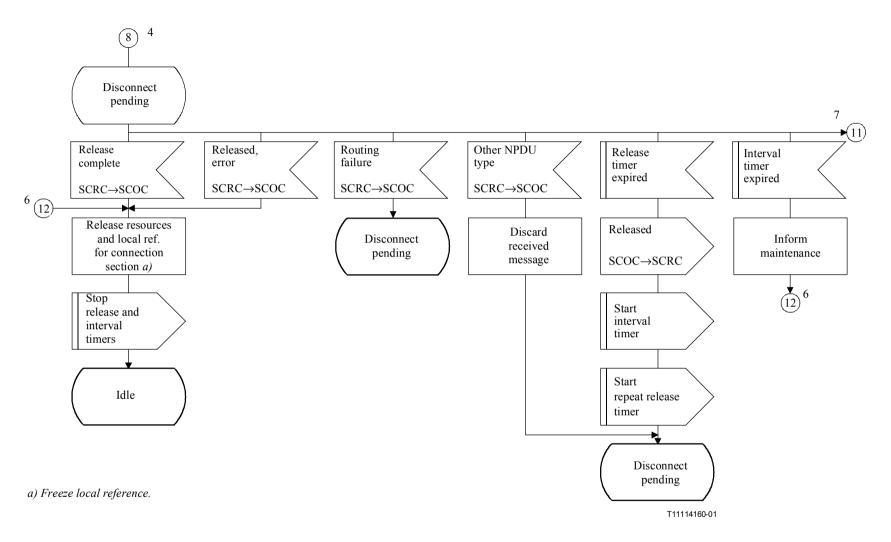
Figure C.2/Q.714 – Connection release procedures at originating node for SCCP connection-oriented control (SCOC) (sheet 6 of 7)
