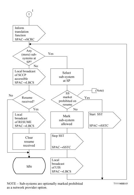
Figure D.3/Q.714 – Signalling point allowed control (SPAC) (sheet 2 of 2)
