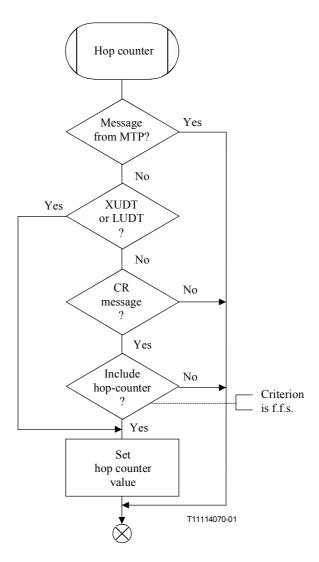
Figure C.1/Q.714 – SCCP routing control procedures (SCRC) (sheet 9 of 12)
