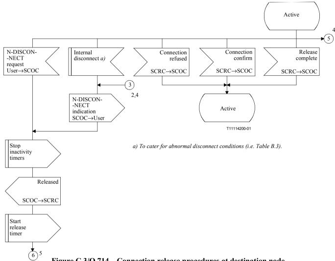
Figure C.3/Q.714 – Connection release procedures at destination node for SCCP connection-oriented control (SCOC) (sheet 3 of 6)
