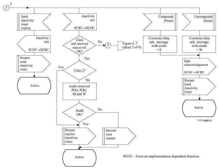
Figure C.8/Q.714 – Data transfer procedures at relay node with coupling for SCCP connection-oriented control (SCOC) (sheet 4 of 4)
