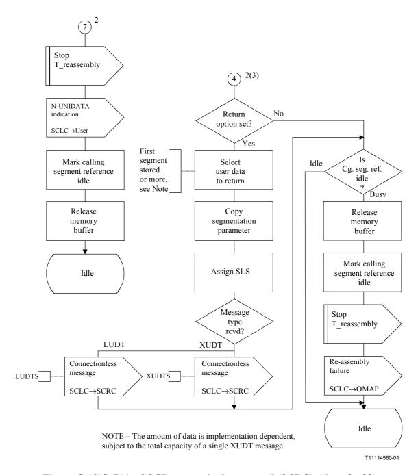
Figure C.12/Q.714 – SCCP connectionless control (SCLC) (sheet 3 of 9)
