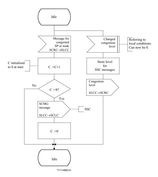
Figure D.12/Q.714 – Local SCCP and nodal congestion control (SLCC) (sheet 1 of 2)
