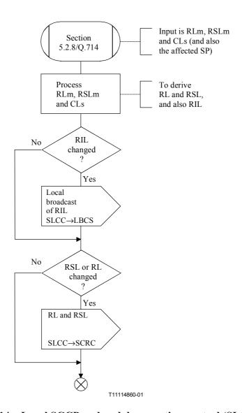
Figure D.12/Q.714 – Local SCCP and nodal congestion control (SLCC) (sheet 2 of 2)
