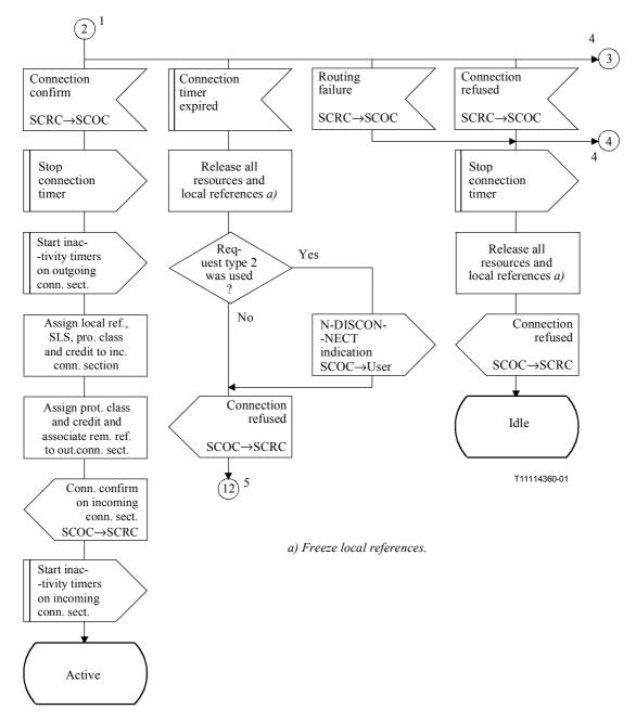
Figure C.7/Q.714 – Connection establishment procedures at relay node with coupling for SCCP connection-oriented control (SCOC) (sheet 3 of 9)
