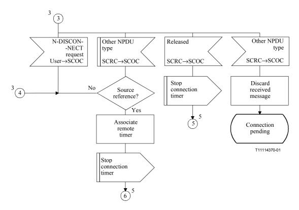
Figure C.7/Q.714 – Connection establishment procedures at relay node with coupling for SCCP connection-oriented control (SCOC) (sheet 4 of 9)
