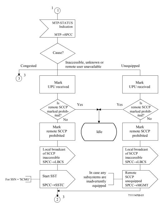
Figure D.4/Q.714 – Signalling point congested control (SPCC) (sheet 2 of 4)
