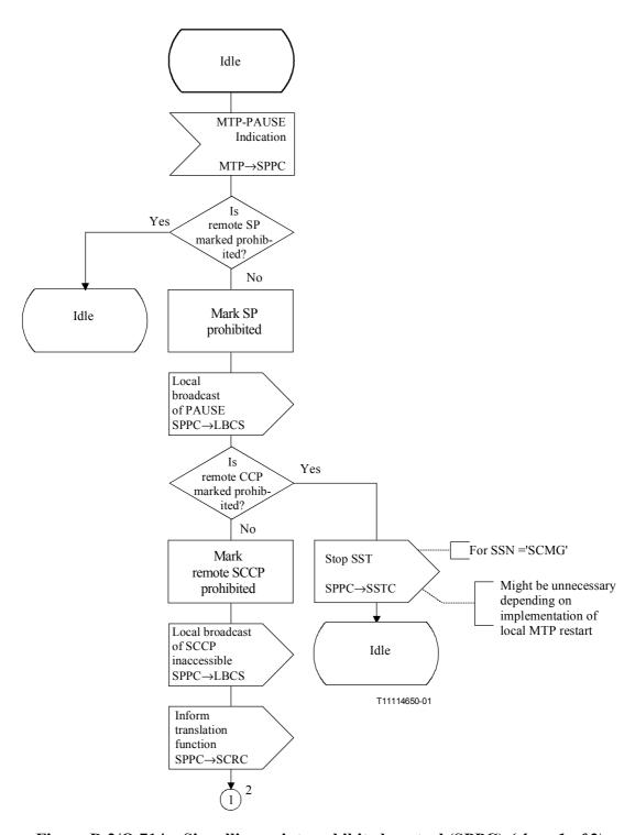
Figure D.2/Q.714 – Signalling point prohibited control (SPPC) (sheet 1 of 2)
