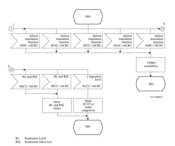
Figure C.1/Q.714 – SCCP routing control procedures (SCRC) (sheet 6 of 12)
