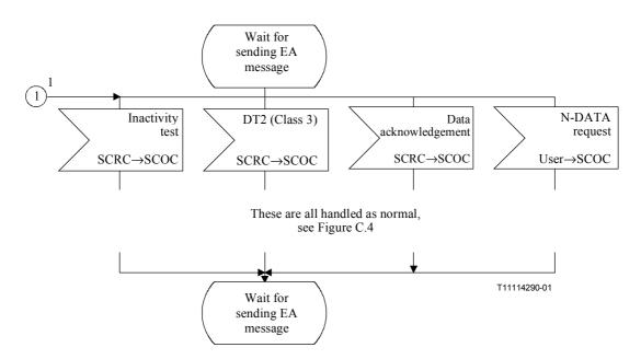
Figure C.5/Q.714 – Expedited data transfer procedures at originating and destination nodes for SCCP connection-oriented control (SCOC) (sheet 2 of 2)
