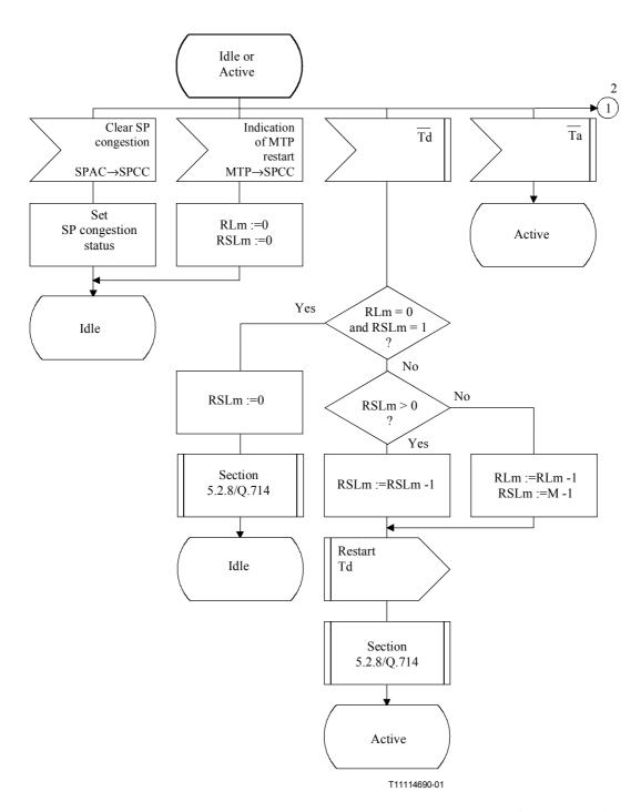
Figure D.4/Q.714 – Signalling point congested control (SPCC) (sheet 1 of 4)
