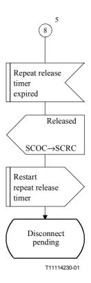
Figure C.3/Q.714 – Connection release procedures at destination node for SCCP connection-oriented control (SCOC) (sheet 6 of 6)
