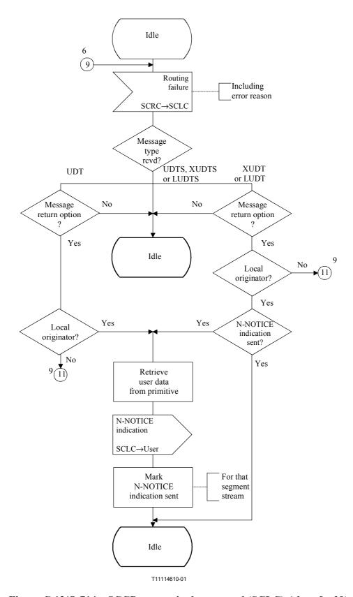
Figure C.12/Q.714 – SCCP connectionless control (SCLC) (sheet 8 of 9)
