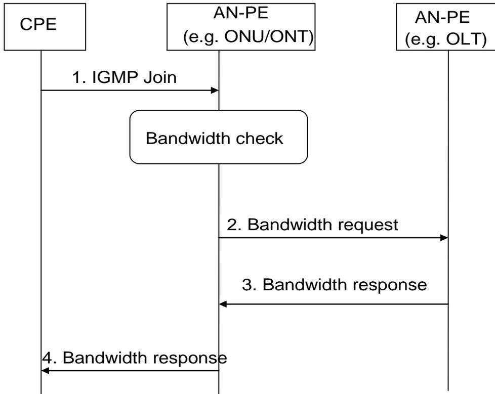
**Figure 9-1 – Multicast admission control procedure when there is sufficient bandwidth in AN-PE**
