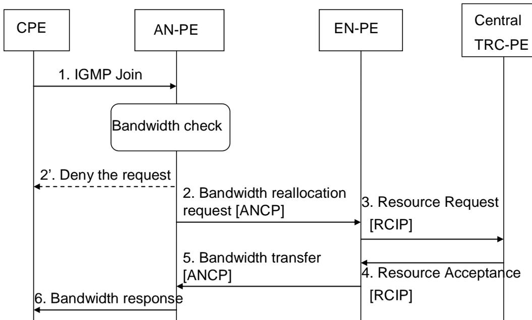
**Figure 9-2 – Multicast admission control procedure when there is no sufficient bandwidth in AN-PE**
