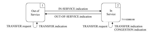
Figure 6-1/Q.2150.1 – State transition diagram for sequences of primitives between the STC and its user
