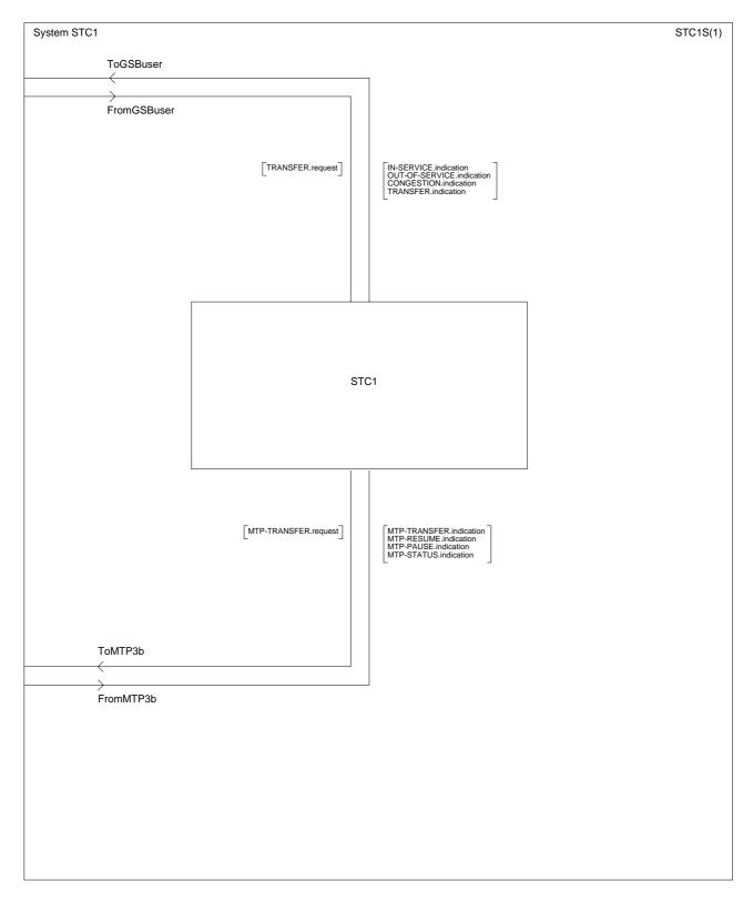
Figure 8-2/Q.2150.1 – SDL system of the AAL type 2 signalling transport converter
