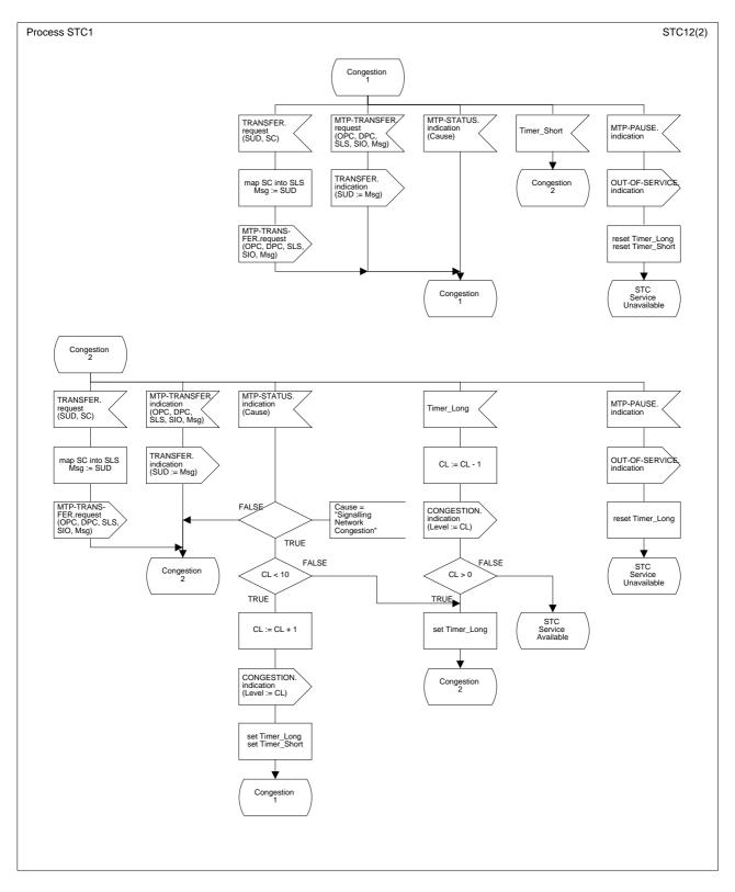
Figure 8-4/Q.2150.1 – SDL diagram for the AAL type 2 signalling transport converter (part 2 of 2)
