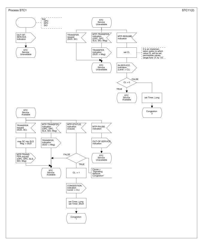
Figure 8-4/Q.2150.1 – SDL diagram for the AAL type 2 signalling transport converter (part 1 of 2)
