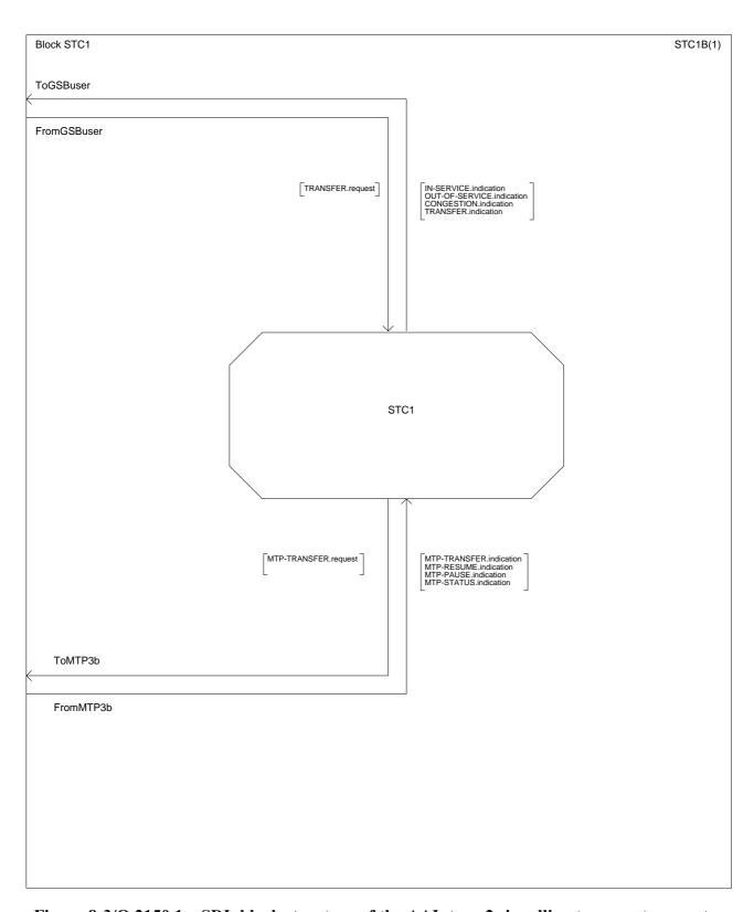
Figure 8-3/Q.2150.1 – SDL block structure of the AAL type 2 signalling transport converter
