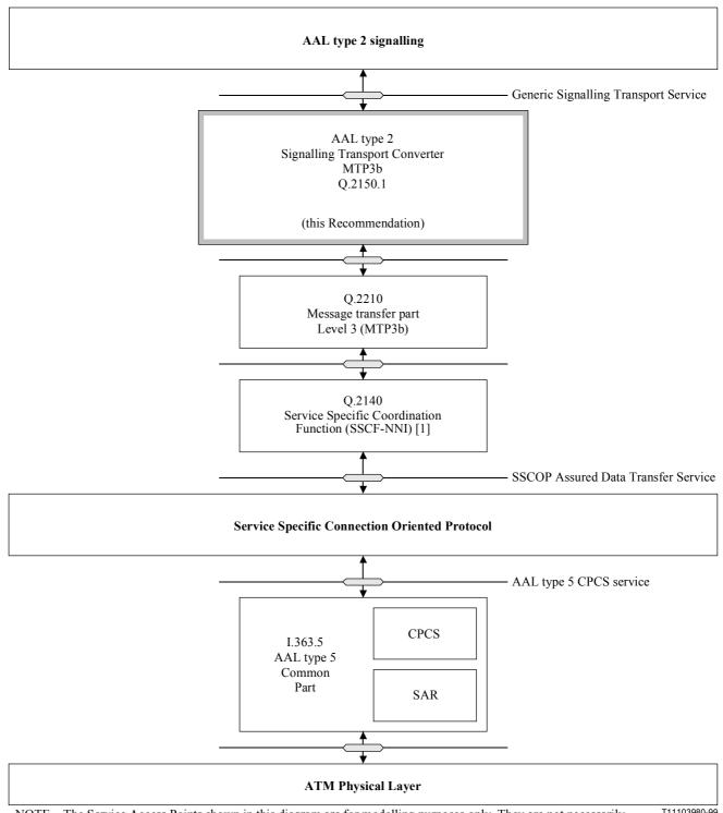
NOTE - The Service Access Points shown in this diagram are for modelling purposes only. They are not necessarily visible or accessible from outside.
