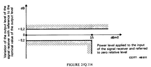
Limits for nonlinear distortion due to the insertion of the signal receiver
