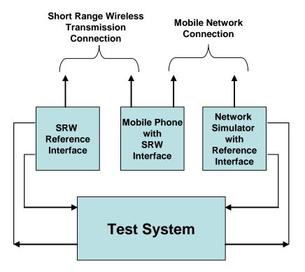
Figure 12-1 – Short range wireless transmission test set-up
