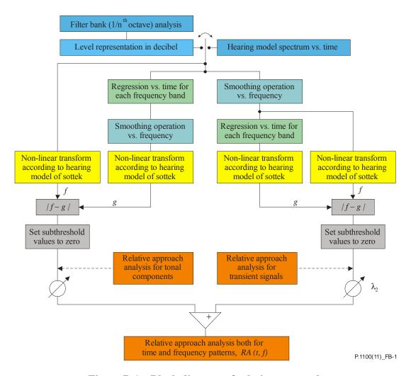
Figure B.1 – Block diagram of relative approach
