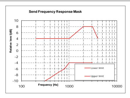
Figure 11-3 – Send frequency response mask (Fig. is informative)
