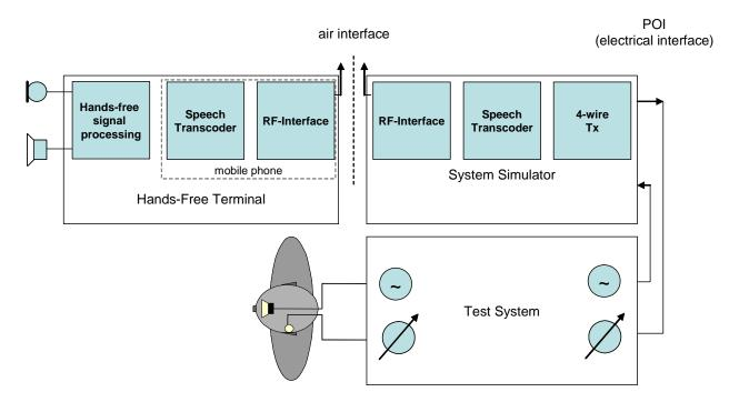
Figure 7-1 – Test arrangement for hands-free terminals
