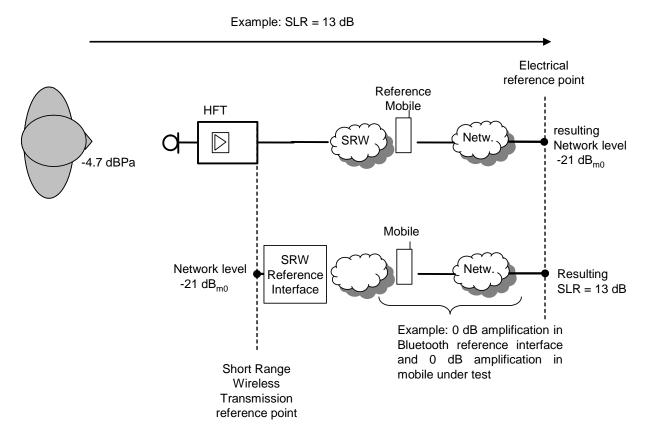
Figure 12-2 – Calibration of the SRW transmission reference interface
