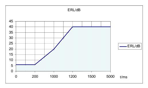
Figure 11-6 – Initial convergence, ERL versus time
