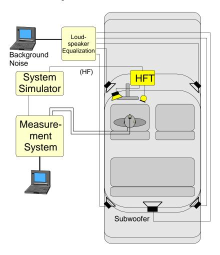
Figure 7-3 – Test arrangement with background noise simulation
