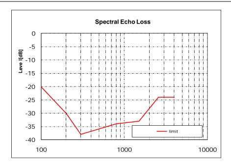
Figure 11-5 – Spectral echo loss mask (Fig. is informative)
