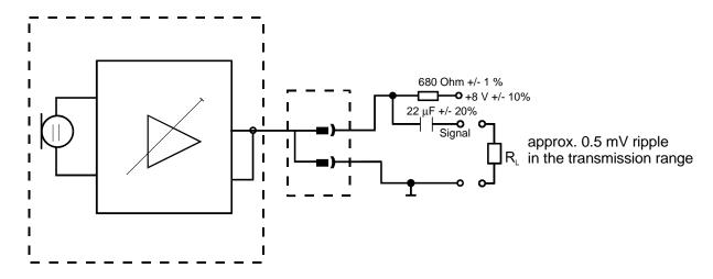
Figure 7-2 – Test arrangement for hands-free microphones and microphone arrangements
