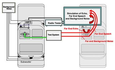
Device under test (DUT, laboratory test set-up) Simulated vehicle at far end
