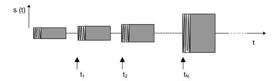
Figure 11-8 – Test signal to determine the minimum activation level and the built-up time
