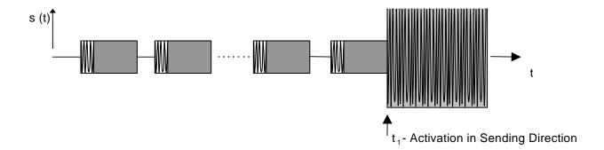
Figure 11-9 – Structure of the test signal for measuring the attenuation range
