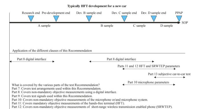
Figure 6-1 – Typical development cycle for a car speakerphone hands-free system and the applicability of the different clauses of this Recommendation during this process
