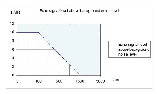
Figure 11-7 – Initial convergence with background noise, requirement on echo signal level versus time
