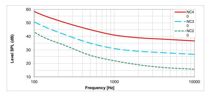
Figure 7-4 – NC-criteria for test environment
