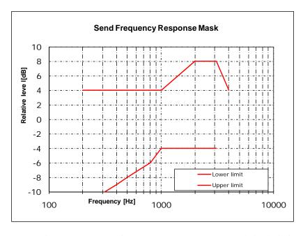
Figure 10-2 – Microphone send frequency response mask (Fig. is informative)
