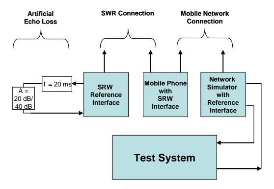
Figure 12-3 – Test set-up with artificial echo loss
