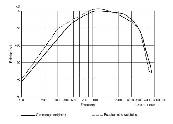
FIGURE A. 1/O.41 Comparison between psophometric and C-message weighting
