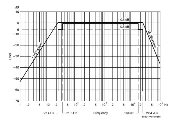
FIGURE 1/0.41 Frequency response characteristics for unweighted measurements
