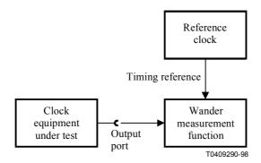
Figure II.3/O.172 – Clock stability measurement configuration
