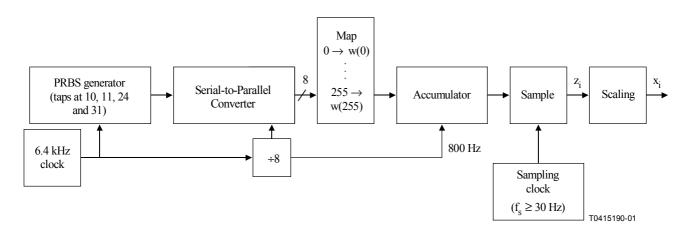
Figure V.2/O.172 – Alternative TIE noise source used for verifying MTIE and TDEV calculation algorithms
