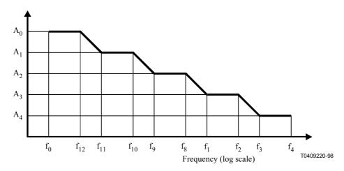
Figure 3/O.172 – Generated jitter/wander amplitude versus jitter/wander frequency
