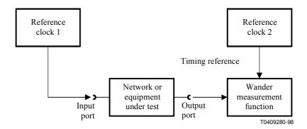
Figure II.2/O.172 – Non-synchronized wander measurement configuration
