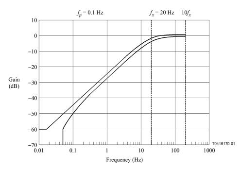
Figure IV.1/O.172 – Mask limits for 2048 kbit/s jitter measurement high-pass filter at 20 Hz
