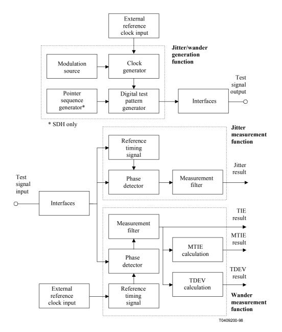
Figure 1/O.172 – Functional block diagram for jitter and wander test set
