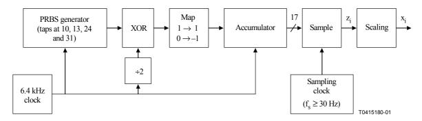
Figure V.1/O.172 – TIE noise source used for verifying MTIE and TDEV calculation algorithms
