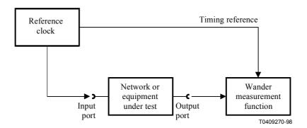
Figure II.1/O.172 – Synchronized wander measurement configuration
