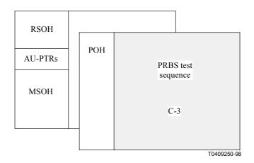
Figure A.2/O.172 – Test signal structure for jitter testing of STM-0 interface
