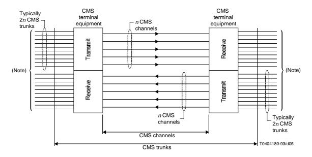
*Note* – CMS trunks are extended, as appropriate, to circuit terminating equipment.
