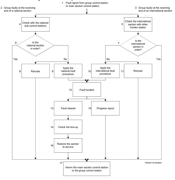
$\label{eq:FIGURE} FIGURE~4/M.2130$  Example of possible action by a frontier station following a fault report
