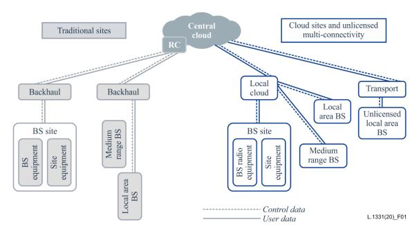
Figure 1 – Network under test definition
