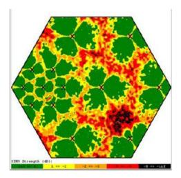
Figure 6 – Typical SINR distribution of a mobile network
