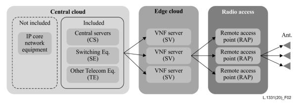
Figure 2 – Generic CRAN architecture layout
