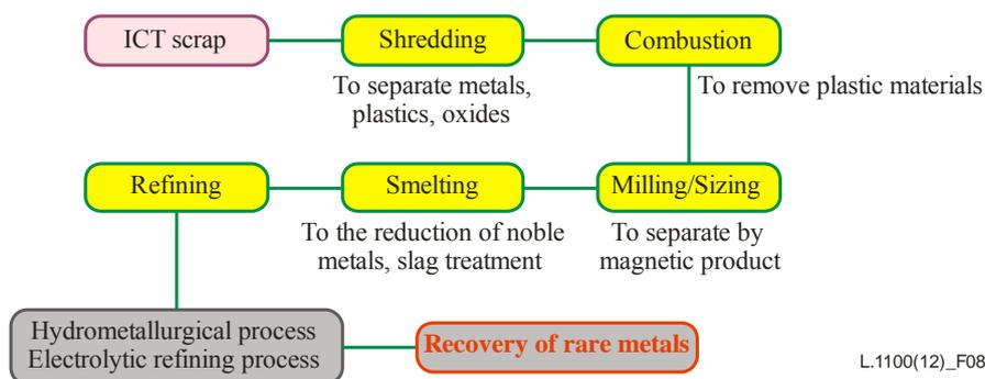
**Figure 8 – A flowchart of recycling process**
