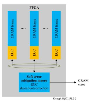
Figure 6.2-2 – Example of soft error reduction macro configuration (See [b-Altera] and [b-Xilinx-WP395])
