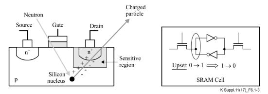
Figure 6.1-3 – Soft error mechanism due to neutron ray in SRAM (See [b-Xilinx-WP395])
