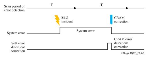
Figure 6.2-3 – Example of an operation when a soft error occurs
