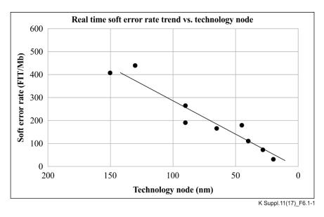
Figure 6.1-1 – Example of CRAM soft error rate vs. feature size (technology node) (See [b-Xilinx-UG116])
