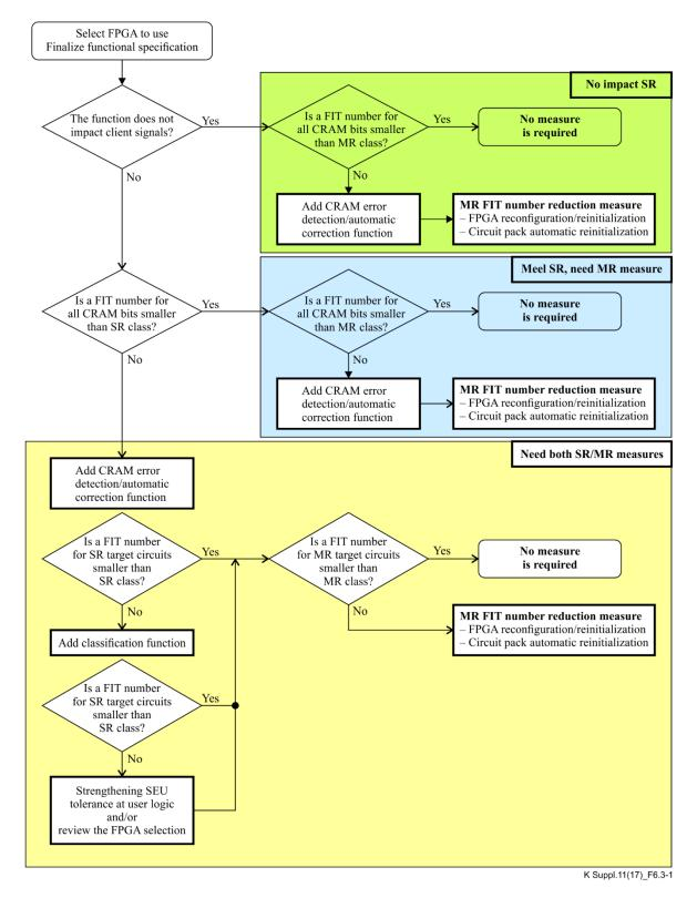
Figure 6.3-1 – Example of a method for improving SR/MR
