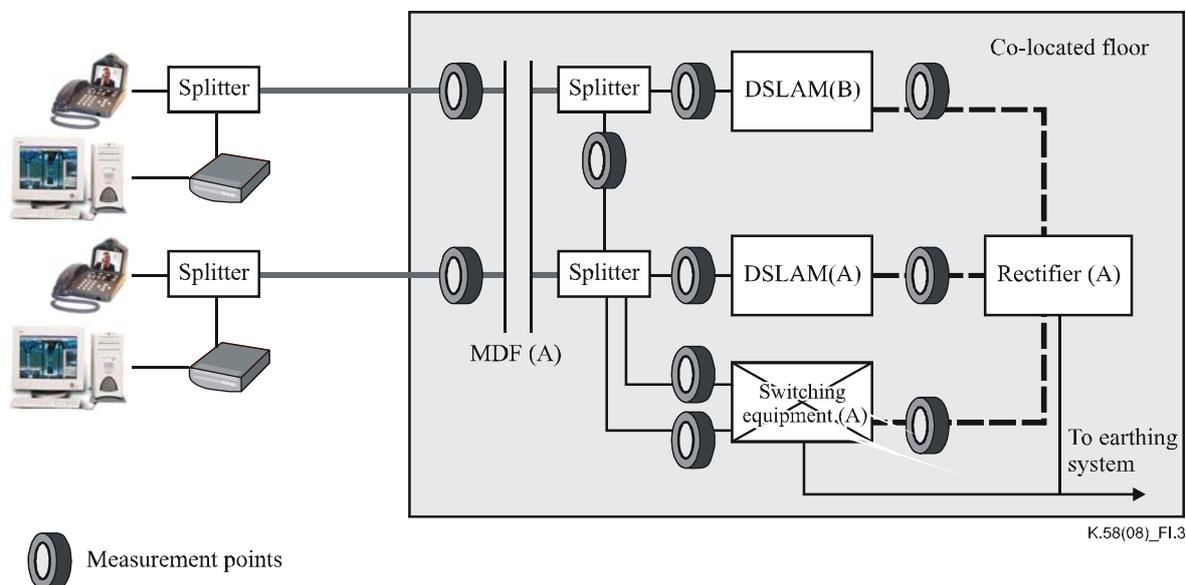
**Figure I.3 – Measurement points**
