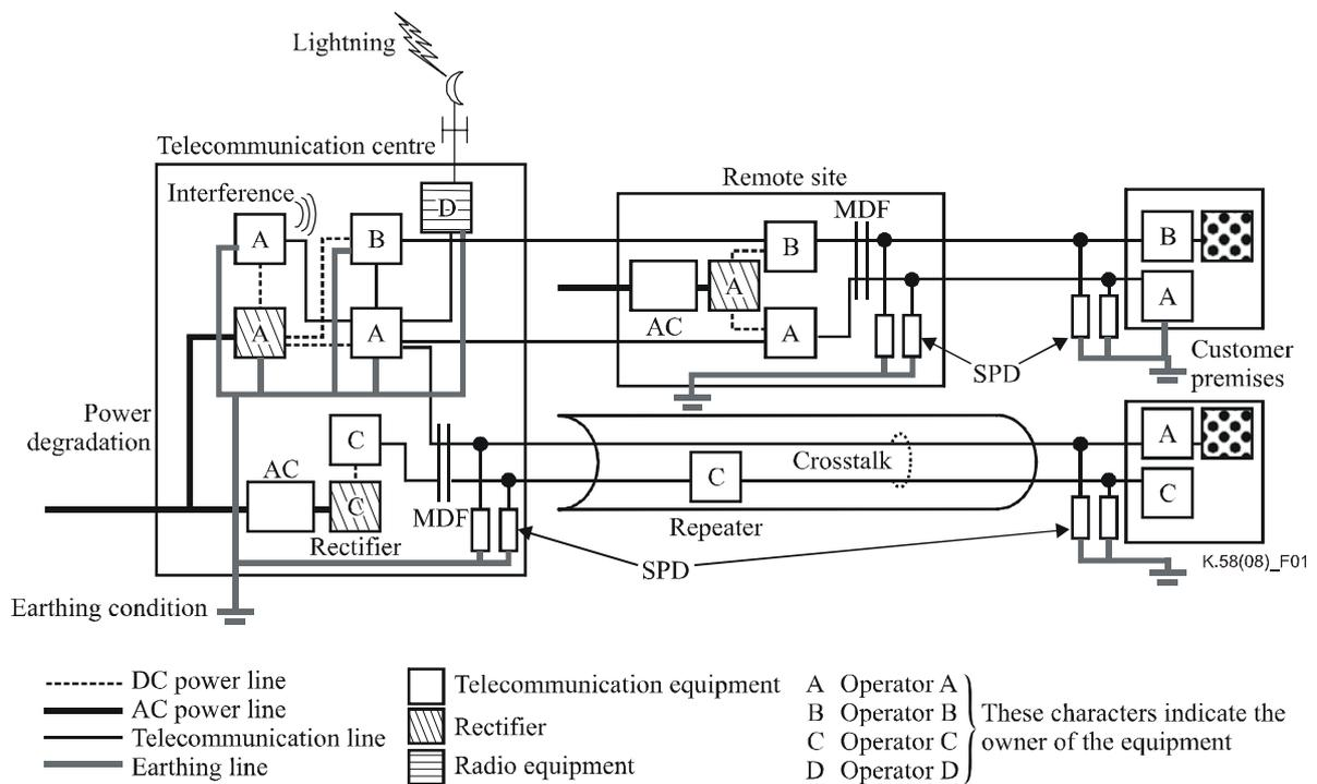
**Figure 1 – An example of a co-located telecommunications installation**
