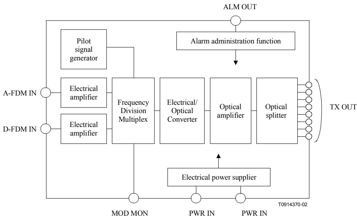
**Figure 4/J.186 – Block diagram of TX**
