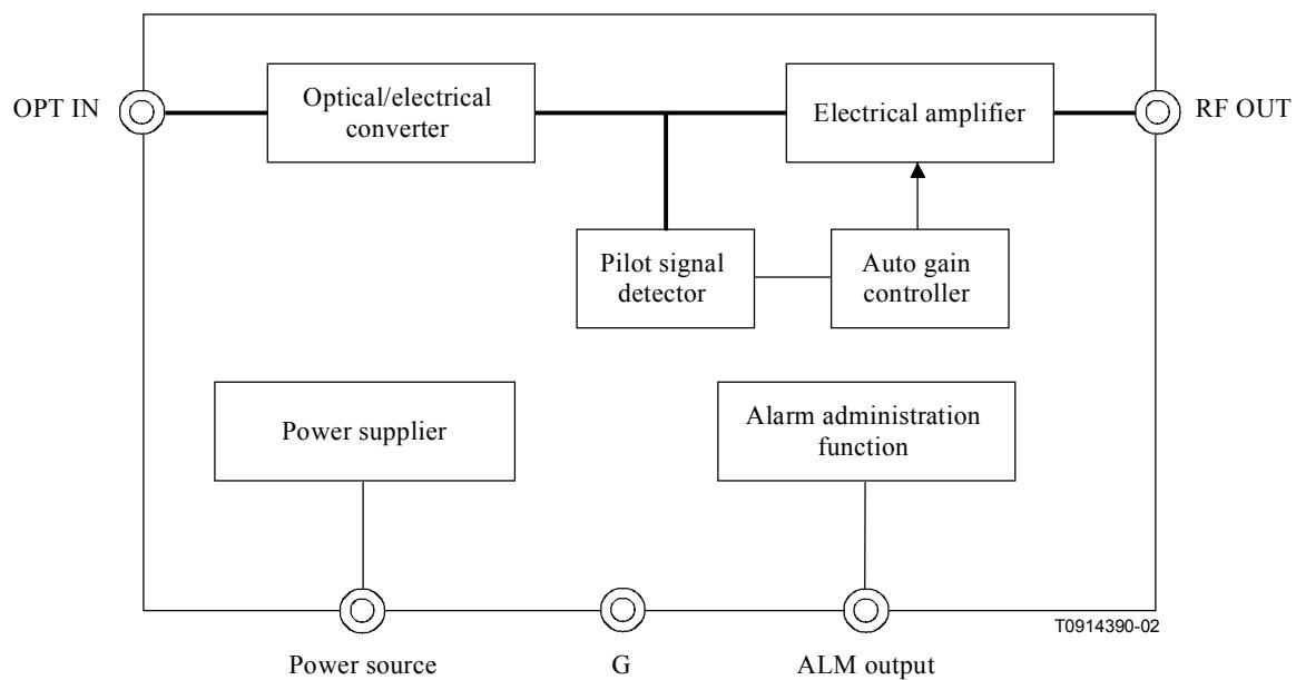
**Figure 6/J.186 – Block diagram of V-ONT**
