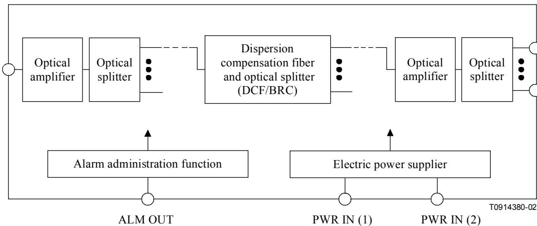
**Figure 5/J.186 – Block diagram of AMP/BRC**
