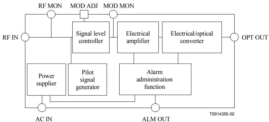
**Figure 2/J.186 – Block diagram of TA**
