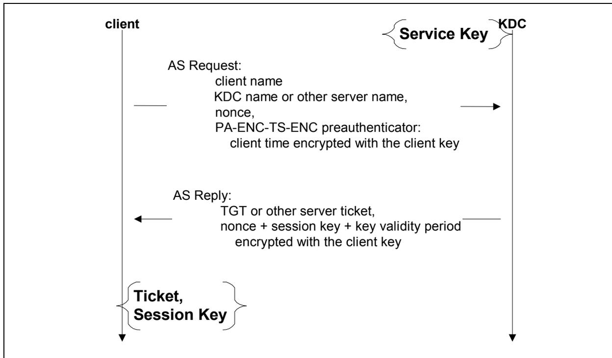
**Figure 6. Symmetric-Key AS Request / AS Reply Exchange**
