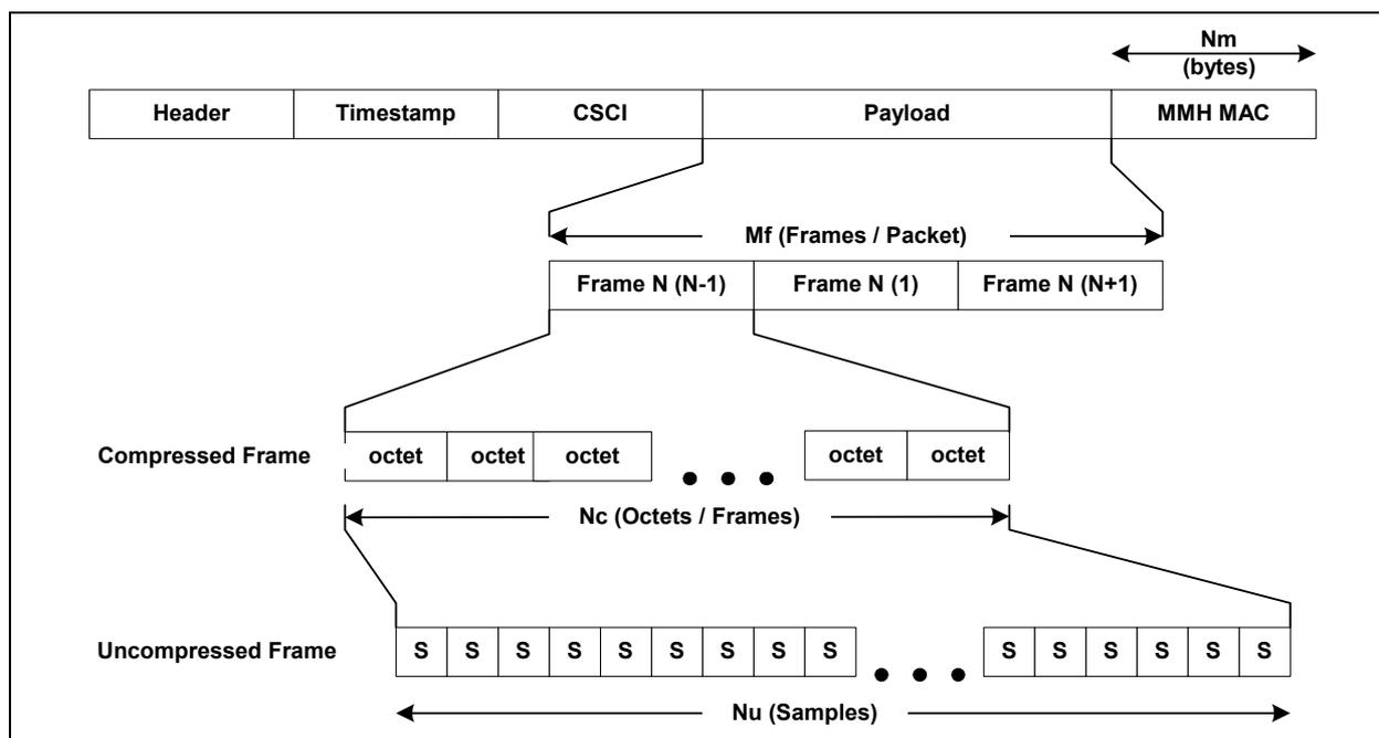
Figure 19. RTP Packet Profile Characteristics
