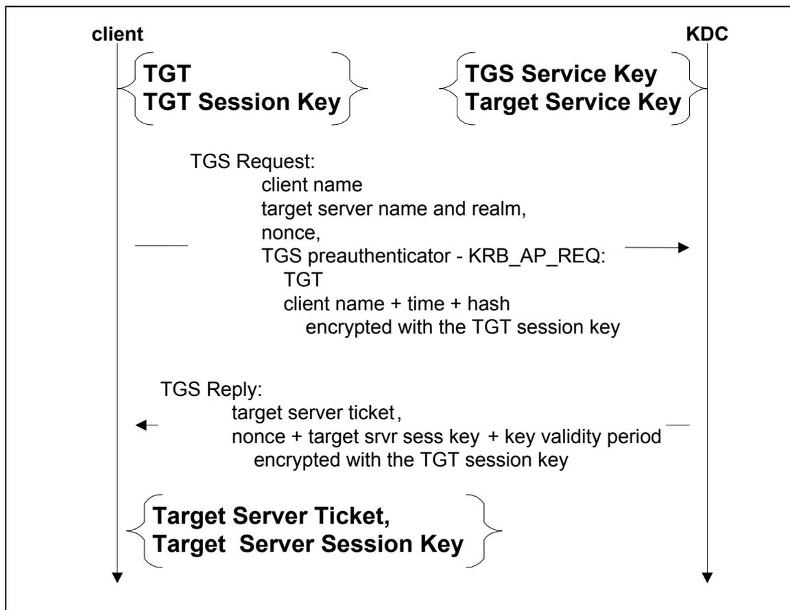
**Figure 7. Kerberos TGS Request / TGS Reply Exchange**
