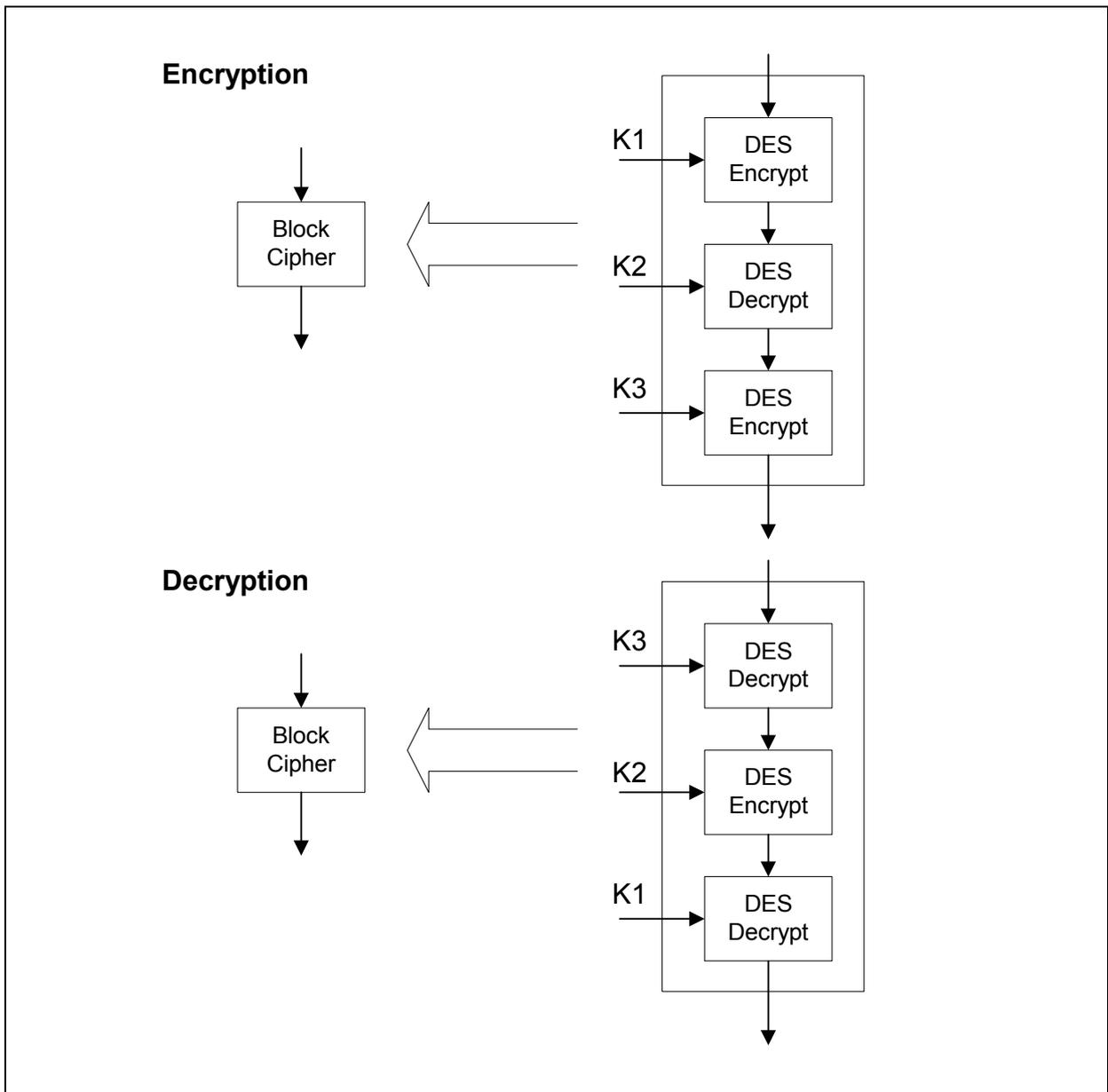
Figure 29. 3DES-EDE as Block Cipher
