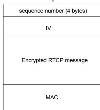
**Figure 21. RTCP Encrypted Packet Format**
