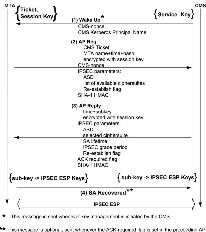
Figure 9. Kerberos AP Request / AP Reply Exchange
