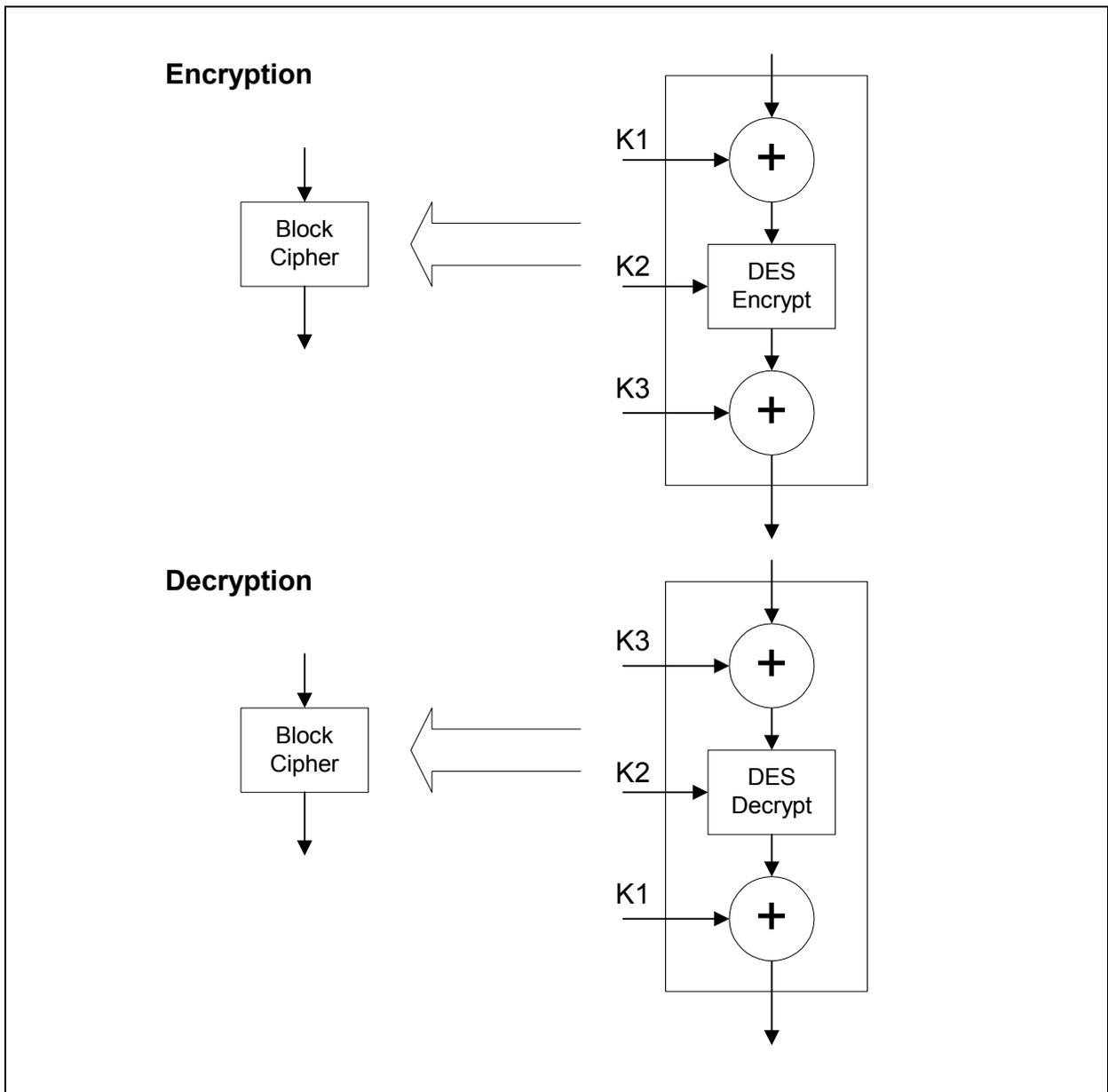
Figure 28. DESX-XEX as Block Cipher
