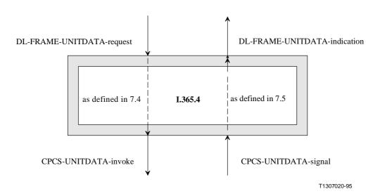
Figure 2/I.365.4 – Relationship of DL-FRAME primitives and AAL type 5 CPCS signals
