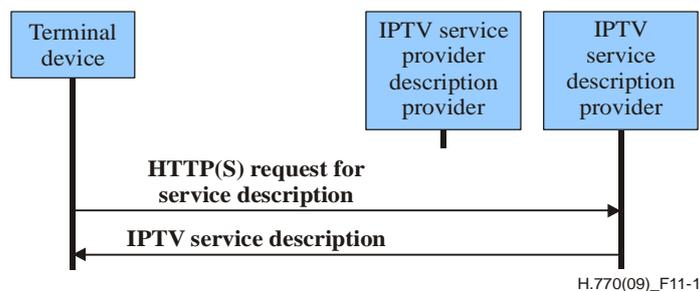
**Figure 11-1 – HTTP or HTTP over TLS request for description of the IPTV services offered by a service provider**
