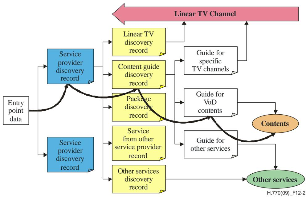
**Figure 12-2 – Example of content selection through a VoD Guide**
