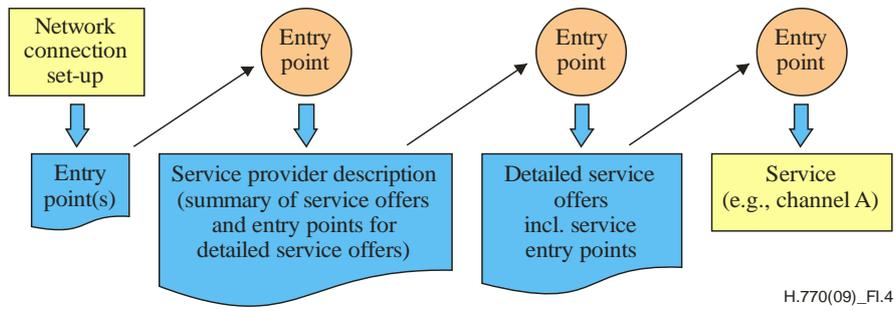
**Figure I.4 – ITU-T H.770 service discovery process**
