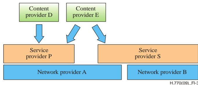
**Figure I.3 – Basic IPTV service provider model**
