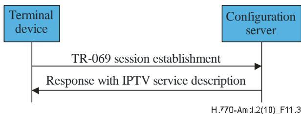
**Figure 11-3 – Using TR-069 to receive the description of the IPTV services**
