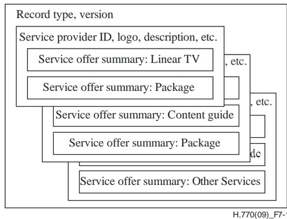
**Figure 7-1 – Graphical representation of the service provider information record**
