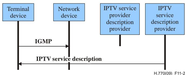
**Figure 11-2 – IGMP or MLD join request to receive the description of the IPTV services offered by a service provider**
