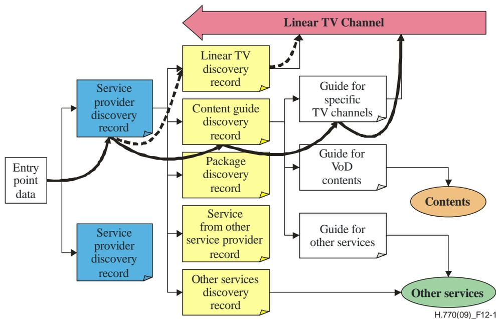
**Figure 12-1 – Example of live channel selection through a service guide**
