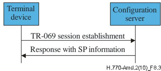
**Figure 8-3 – Using TR-069 to receive the description of the available IPTV service providers**
