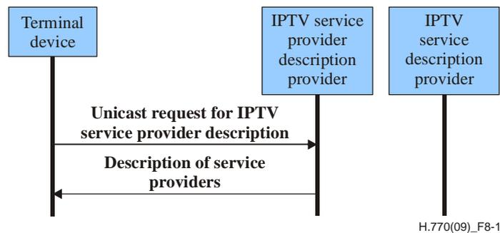
**Figure 8-1 – Unicast request to get the description of the available IPTV service providers**
