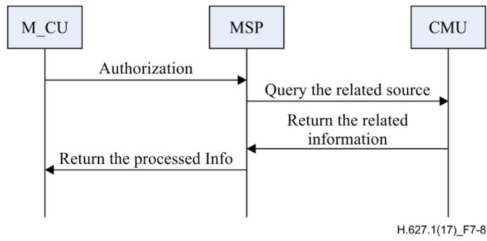
**Figure 7-8 – Procedural flows for querying PU related parameters**
