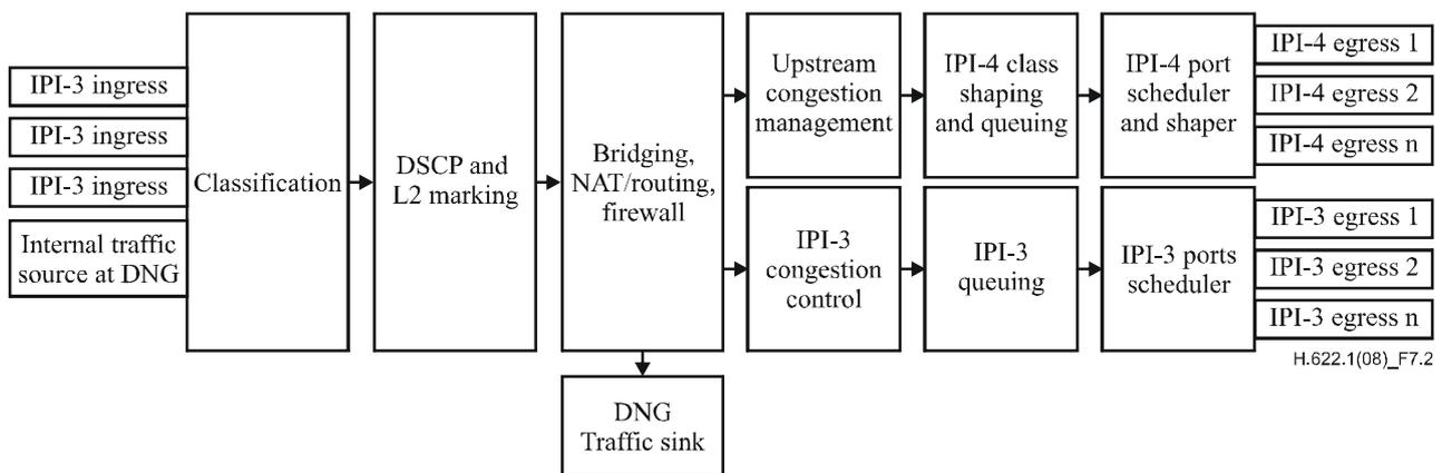
Figure 7-2 – QoS functions from IPI-3 interfaces
