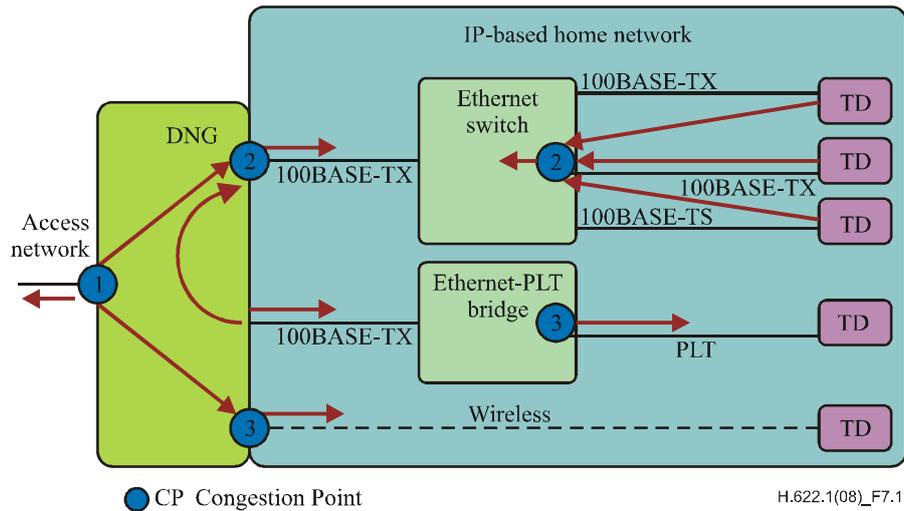
**Figure 7-1 – Potential congestion points in a typical home network**
