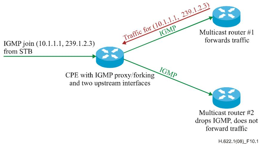
**Figure 10-1 – IGMP proxy in forking mode**
