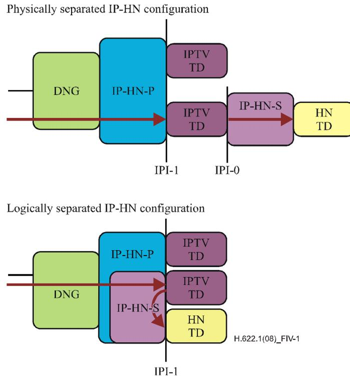
**Figure IV.1 – Example configurations for an IP-based home network**
