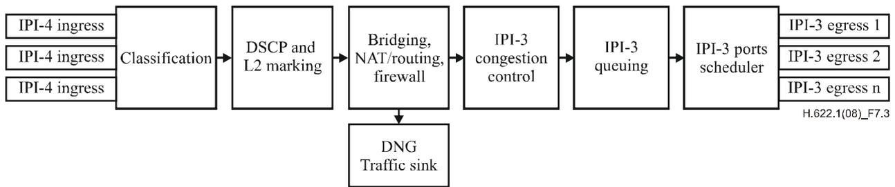
**Figure 7-3 – QoS functions from IPI-4 interface**
