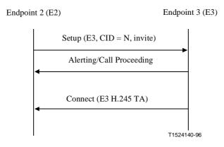
Figure 27/H.323 – MC invite signalling
