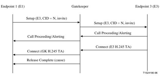
Figure 31/H.323 – Gatekeeper routed invite signalling
