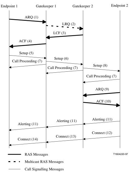
Figure 24/H.323 – Optional Called Endpoint Signalling
