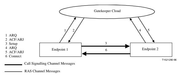
Figure 10/H.323 – Direct endpoint call signalling
