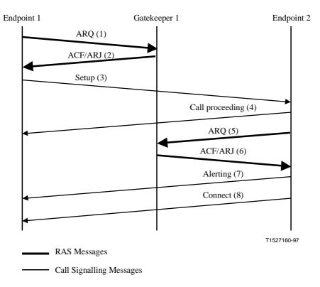
Figure 14/H.323 – Both endpoints registered, same Gatekeeper – Direct call signalling
