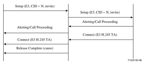
Figure 28/H.323 – Non-MC invite signalling
