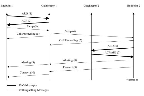
Figure 22/H.323 – Both endpoints registered – Routed/direct call signalling
