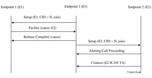
Figure 30/H.323 – Non-MC join signalling
