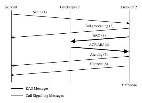
Figure 18/H.323 – Only called endpoint registered – Direct call signalling
