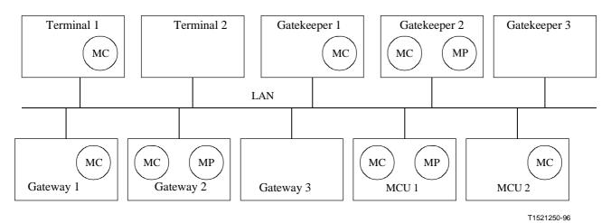
NOTE – Gateway, Gatekeeper and MCU can be a single device.
