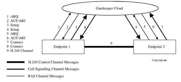
Figure 11/H.323 – Direct H.245 control channel connection between endpoints
