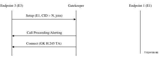
Figure 32/H.323 – Gatekeeper routed join signalling
