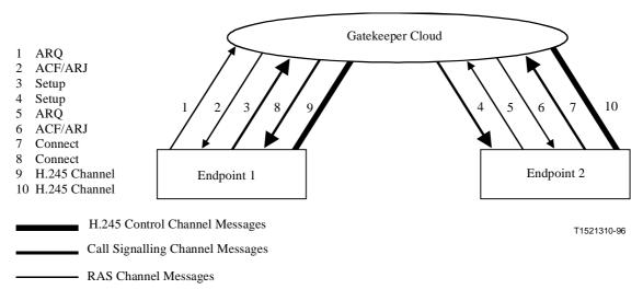
Figure 12/H.323 – Gatekeeper routed H.245 control
