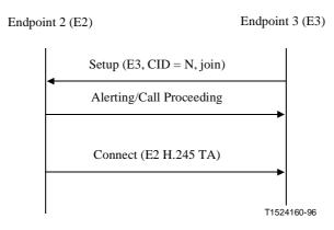
Figure 29/H.323 – MC join signalling
