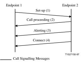
Figure 13/H.323 – Basic call setup, no Gatekeepers
