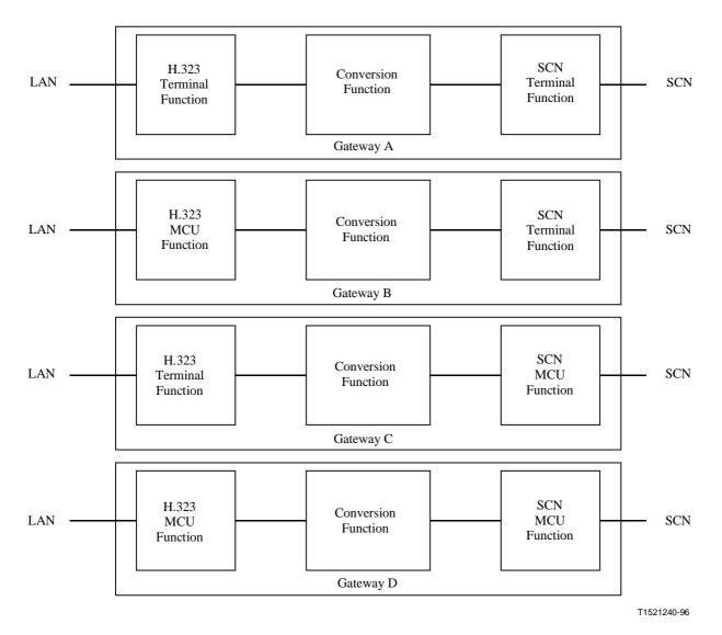
Figure 5/H.323 – H.323 gateway configurations
