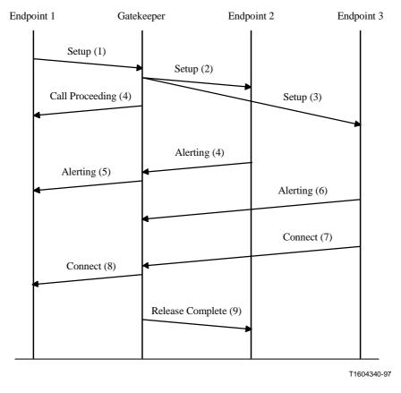
Figure III.2/H.323 – Example of user location using H.225/Q.931 signalling (RAS signalling not shown for clarity)
