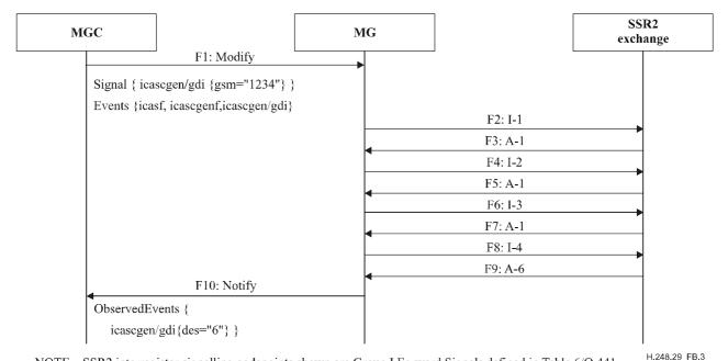
NOTE – SSR2 interregister signalling codepoints shown are Group I Forward Signals defined in Table 6/Q.441, and Group A Backward Signals defined in Table 8/Q.441.
