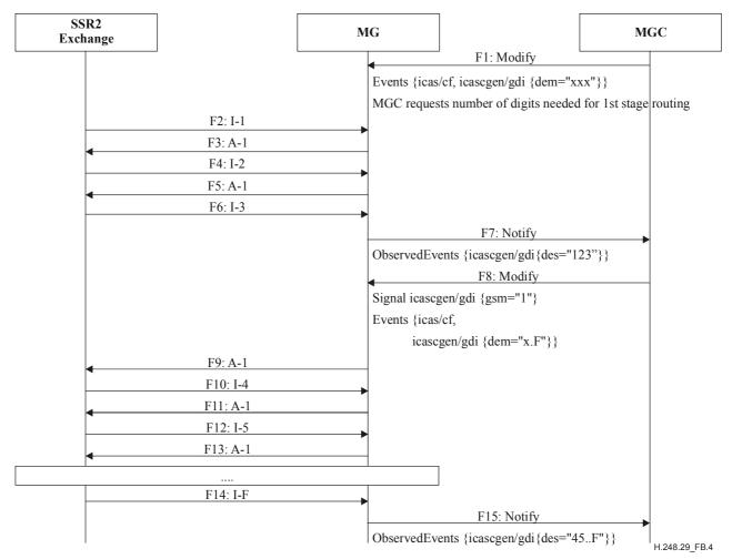
NOTE – SSR2 interregister signalling codepoints shown are Group I Forward Signals defined in Table 6/Q.441, and Group A Backward Signals defined in Table 8/Q.441.
