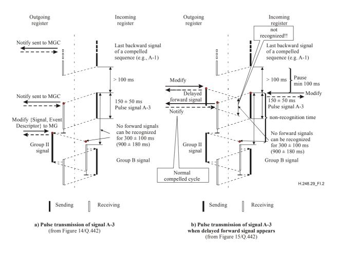
Figure I.2/H.248.29 – Time sequence of a pulsed transmission signal based on ITU-T Q. Suppl. 7
