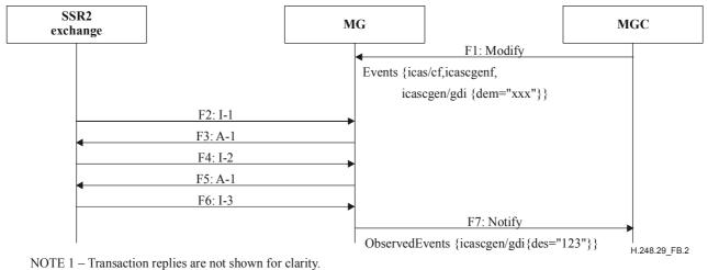
NOTE 2 – SSR2 interregister signalling codepoints shown are Group I Forward Signals defined in Table 6/Q.441, and Group A Backward Signals defined in Table 8/Q.441.
