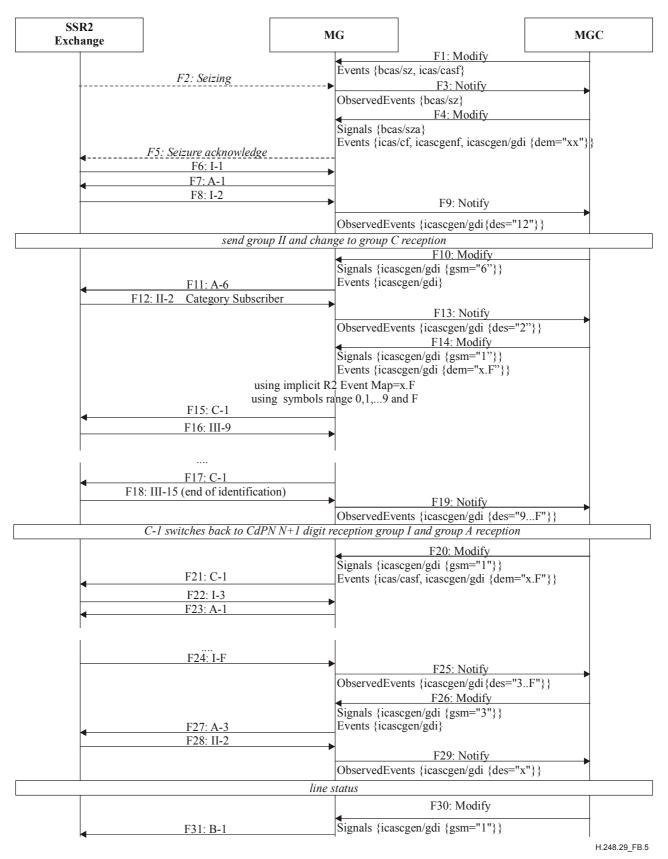
NOTE – SSR2 interregister signalling codepoints used here are Group II Forward Signals defined in Table 7/Q.441, Group III Forward Signals and Group C Backward Signals to show an example of national extensions. The exact definitions of these codepoints are not relevant here.
