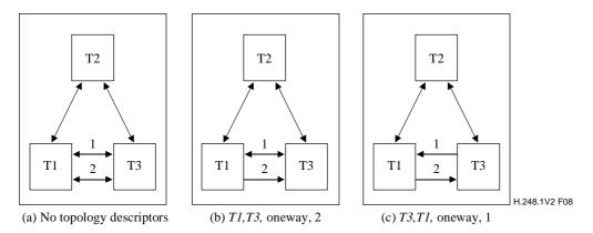
Figure 8/H.248.1 – Example Topology at stream level
