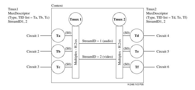
Figure 5/H.248.1 – Multiplexed termination scenario – Circuit-to-circuit
