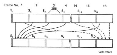
$\begin{array}{l} \mathbf{S_1} \ \mathbf{S_3} \ \mathbf{S_5} \ \mathbf{S_7} \ \mathbf{S_9} \ \mathbf{S_{11}} \, \mathbf{S_{13}} = 0001101 \\ \mathbf{S_{15}} \ \ \text{Multiframe alignment signal} \\ \mathbf{S_2} \ \mathbf{S_4} \ \mathbf{S_6} \ \dots \mathbf{S_{16}} \ \ \text{Control information} \end{array}$
