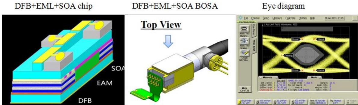
**Figure 8-32 – Schematic of EML transmitter with SOA integrated on the laser chip**
