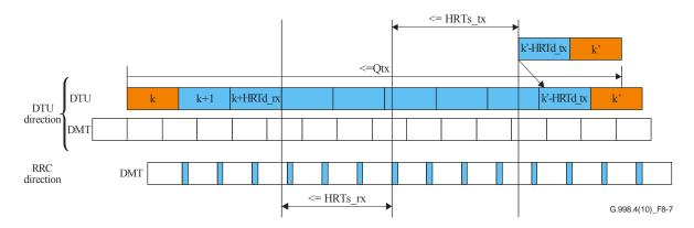
Figure 8-7 – Relationship between half roundtrip definition and minimal  $Q_{tx}$
