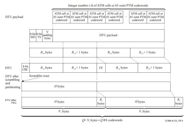
Figure 8-4 – Example of structure of DTU with CRC at the head (Framing type 4, W=2) and synchronization with RS codewords  $[M_1=2, \underline{T}_1=Q=2, SEQ_1=2, \text{ and } B_{10}=(H/2)-1]$
