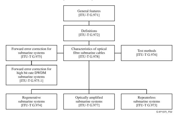
Figure 2 – Relationships amongst Recommendations relevant to optical submarine cable systems
