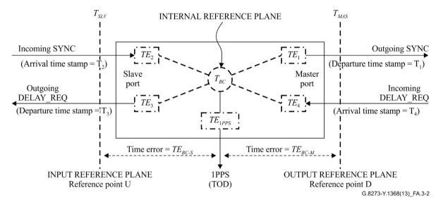
Figure A.3-2 – Time error generation components in a boundary clock
