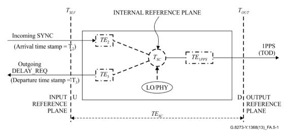
Figure A.5-1 – Time error generation components in a slave clock
