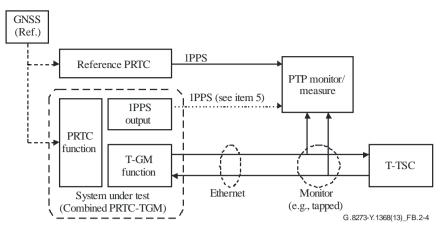
Figure B.2-4 – Passive measurement set-up for a combined "PRTC + T-GM"
