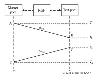
Figure A.1-1 – Depicting the situation where the system under test (SUT) is connected to a test device and PTP messages are exchanged
