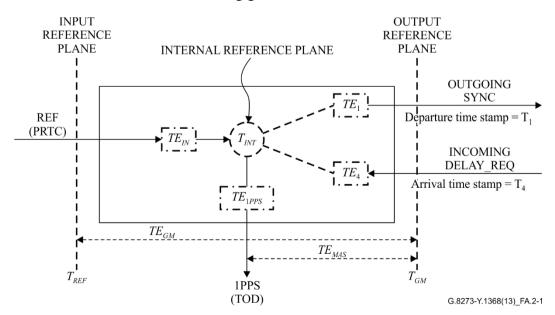
Figure A.2-1 – Noise generation model for a grandmaster clock
