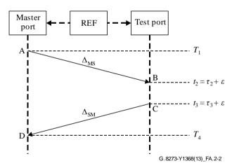
Figure A.2-2 – Depicting the situation where the SUT is connected to test device and PTP messages are exchanged
