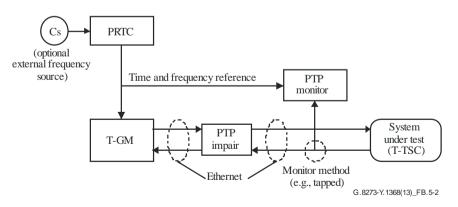
Figure B.5-2 – Measurement set-up for systems with T-TSC based on packet timing signal
