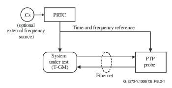
Figure B.2-1 – Active measurement set-up for (PTP) telecom grandmaster
