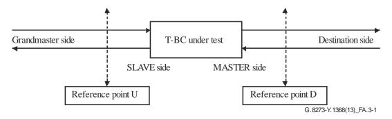
Figure A.3-1 – Demarcation of measurement points for testing BC performance
