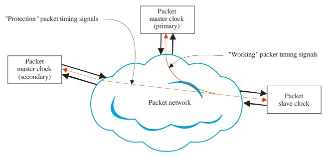
NOTE – For clarity, the network reference signals to masters are not shown.
