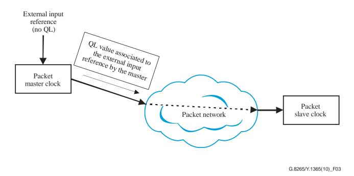
Figure 3 – Example of use case where forcing the QL value at the input of the PTPv2 master is needed
