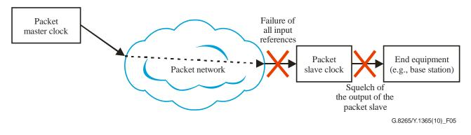
**Figure 5 – Squelching at output of packet slave**
