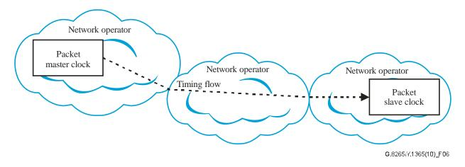
**Figure 6 – Packet timing flow over partitioned network**
