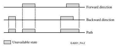
Figure A.2 – Example of the unavailable state of a path
