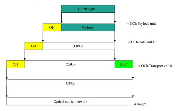
Figure 1 – OTN signal structure
