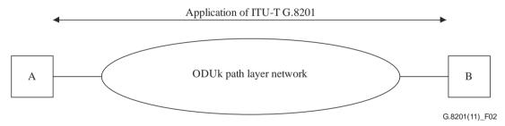
NOTE – A and B are path end points located at the path terminations as defined in [ITU-T G.798].
