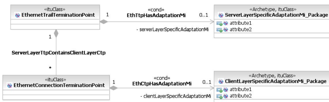
Figure 5-6 – Illustrative diagram for MPLS-TP server adaptation modelling
