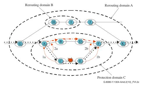
Step 1: The protection mechanism is coordinated between node A and node F in protection domain C after a failure of working path.
