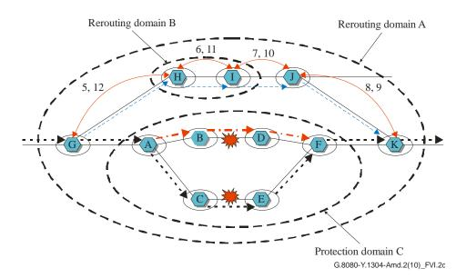
Figure VI.2 – Signalling flow of combination of protection and restoration
