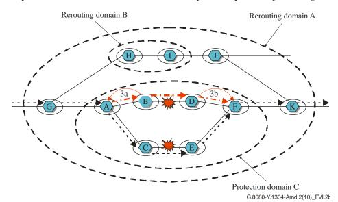
Step 2: Both node A and node F receive a failure notify after the protection path fails again.
