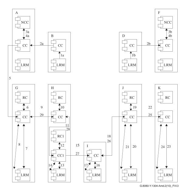
Figure VI.3 – Component interactions of combination of protection and restoration
