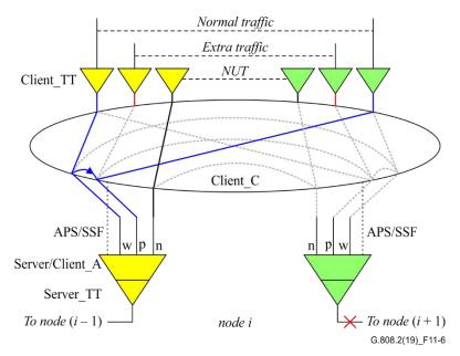
Figure 11-6 – Functional model of a node adjacent to a failure in short wrapping protection on a SLRing
