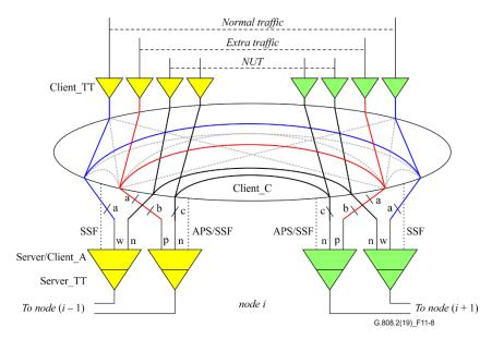
Figure 11-8 – Dedicated section link ring protection functional model
