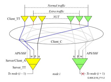
Figure 11-2 – Functional model of a node adjacent to a failure in wrapping protection on a SLRing
