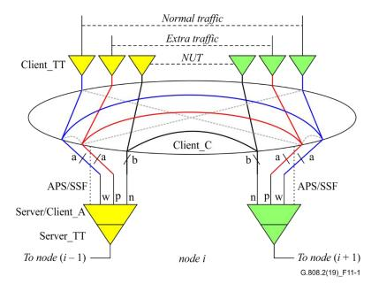
Figure 11-1 – Shared section link ring protection functional model
