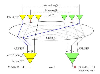
Figure 11-4 – Functional model of an ingress or egress node of normal traffic signal in steering protection on a SLRing
