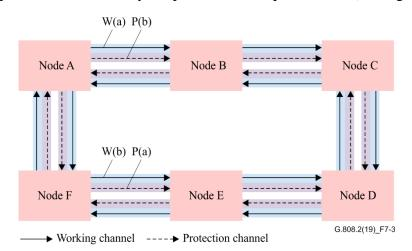
Figure 7-3 – Working transport entity and protection transport entity in dedicated section link ring protection
