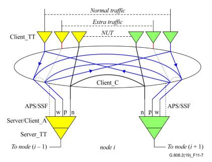
Figure 11-7 – Functional model of an intermediate node in short wrapping protection on a SLRing
