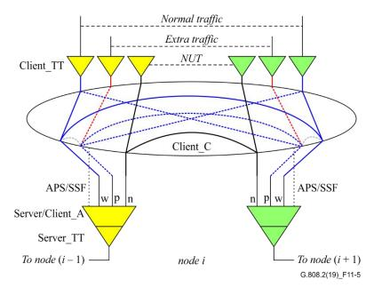
Figure 11-5 – Functional model of an intermediate node in steering protection on a SLRing
