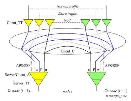
Figure 11-3 – Functional model of an intermediate node in wrapping protection on a SLRing
