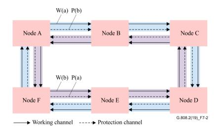
Figure 7-2 – Working transport entity and protection transport entity in shared section link ring protection
