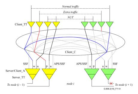
Figure 11-9 – Functional model of a node adjacent to a failure in span switch protection on a DLRing
