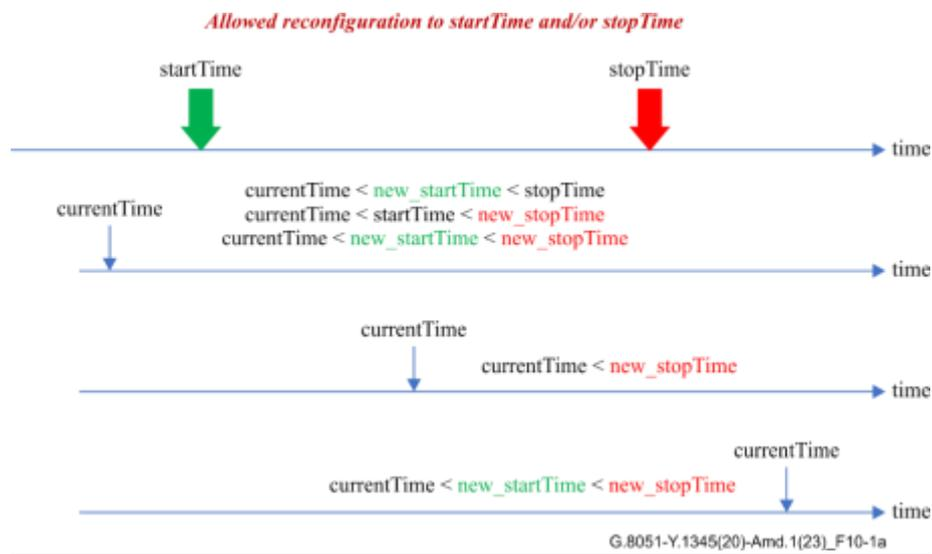
**Figure 10-1a – Allowed reconfiguration to start<sub>Time</sub> and/or stop<sub>Time</sub>**
