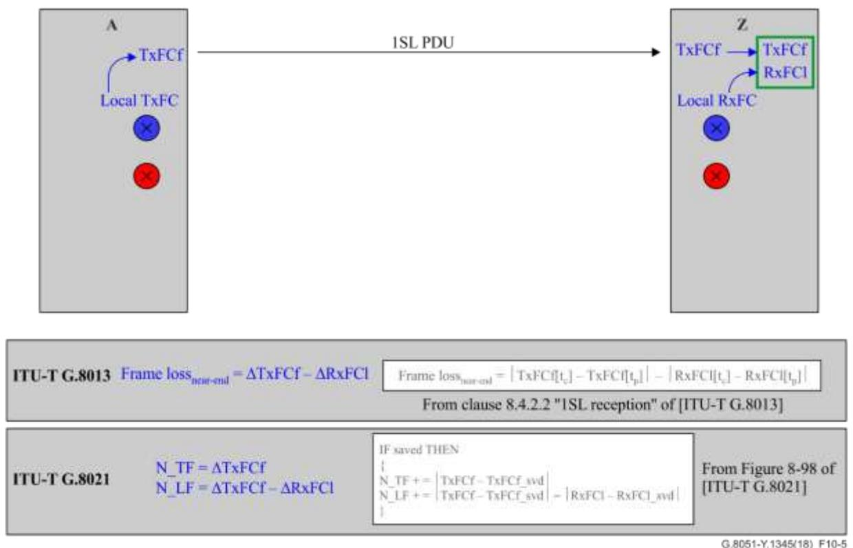
**Figure 10-5 – Dual-ended loss measurement using 1SL**
