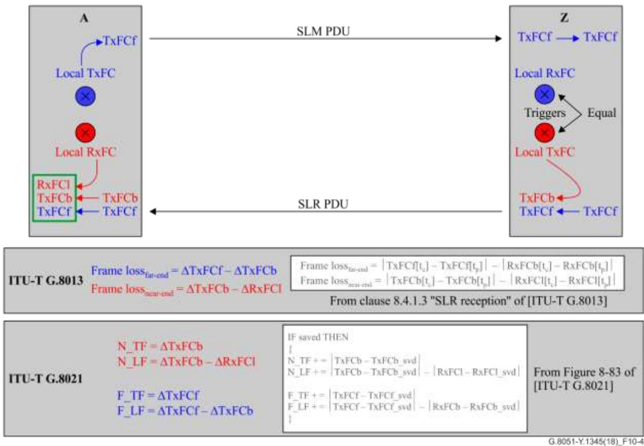
**Figure 10-4 – Single-ended loss measurement using SLM/SLR**
