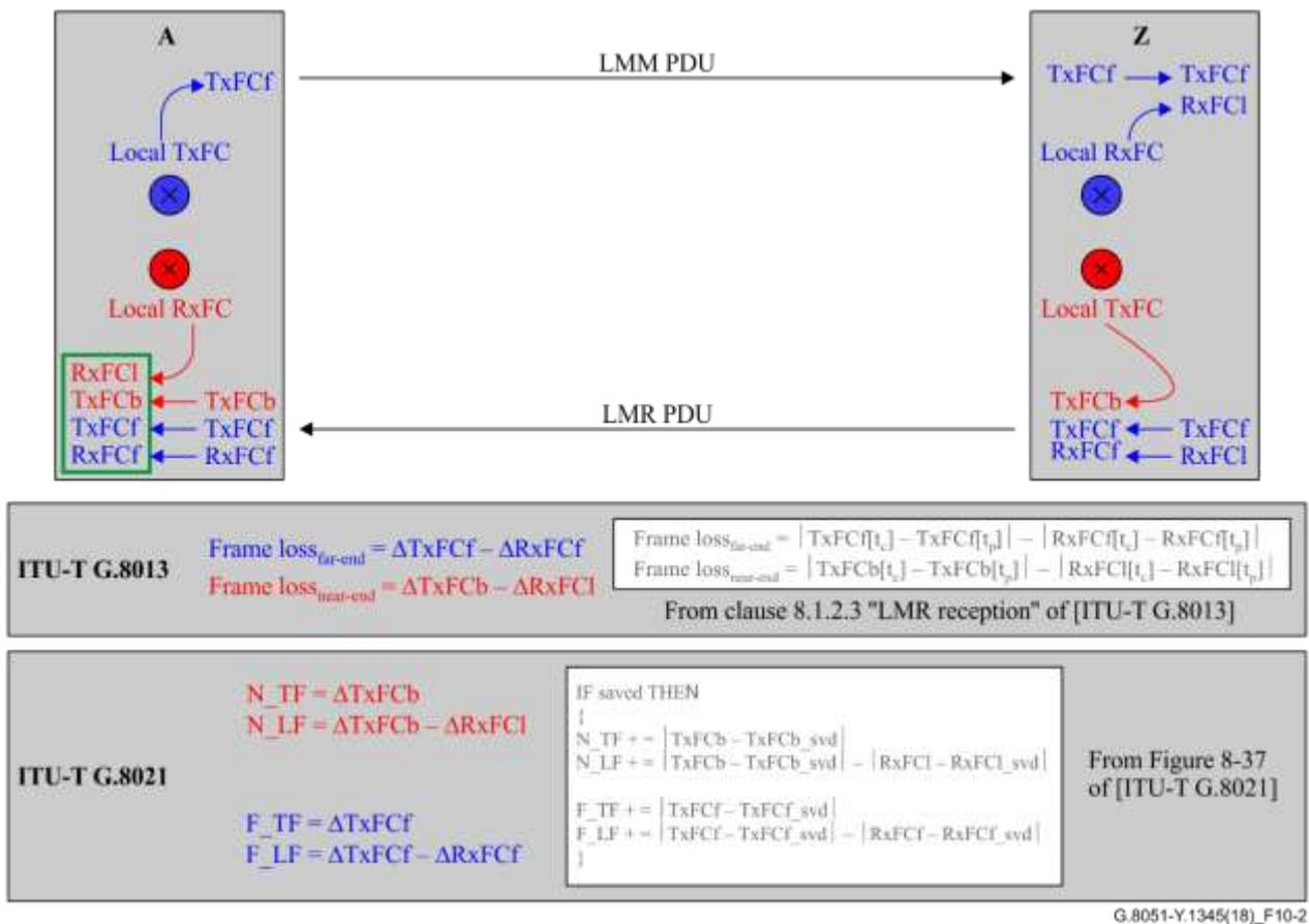
Figure 10-2 – Single-ended loss measurement using LMM/LMR
