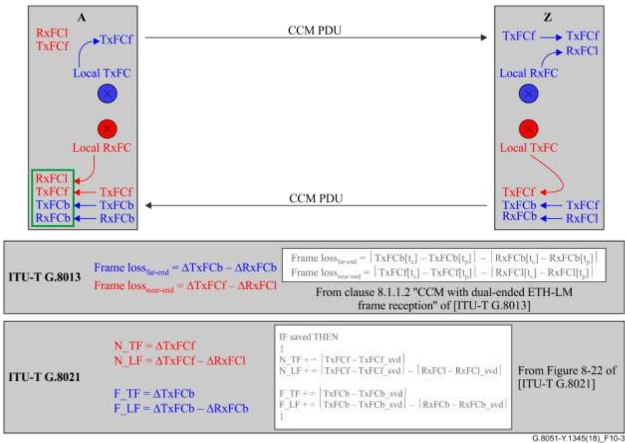
**Figure 10-3 – Dual-ended loss measurement using CCM**
