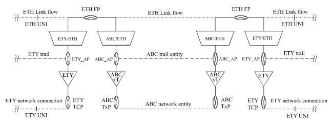
ABC - a connection oriented circuit switched or connection oriented packet switched or connectionless technology
