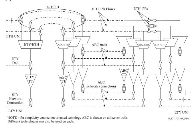
Figure 8-1/G.8011/Y.1307 – Network portion of the multiplexed access line topology
