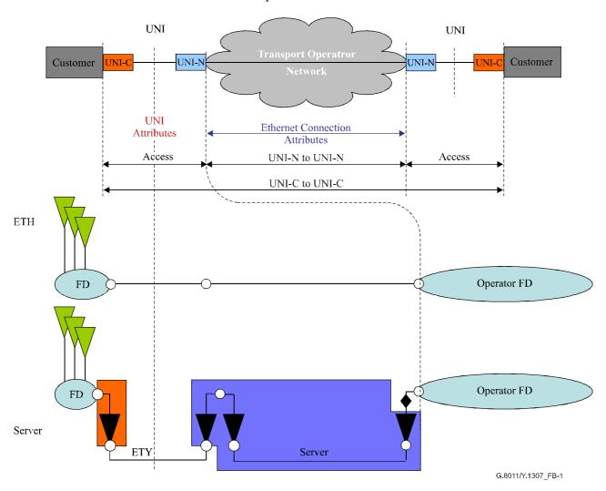
Figure B.1/G.8011/Y.1307 – Single provider view of Ethernet service areas with distributed UNI-N
