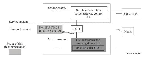
Figure 1 – IP-to-IP voice gateway in the NGN functional architecture
