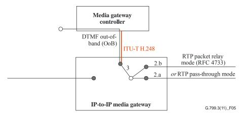
Figure 5 – Interworking between user and control plane interfaces of the IP-to-IP voice gateway
