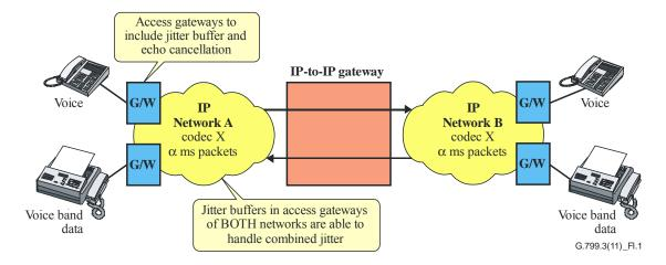
Figure I.1 - Scenario 1: Same codec, same packet size, no jitter buffer
