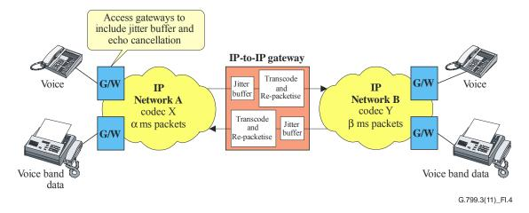
Figure I.4 – Scenario 4: Different codec, different packet size
