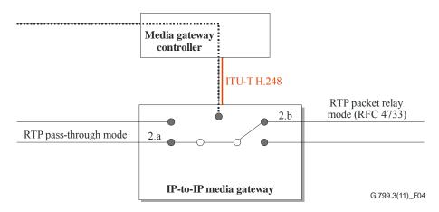
Figure 4 – Interworking between a "pass-through" and a "packet relay" domain
