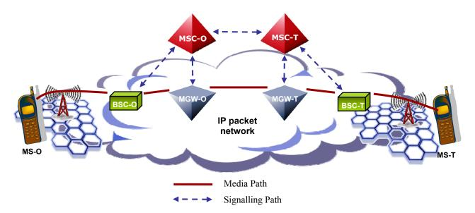
Figure I.1 – Mobile-mobile non-transcoder free operation VoIP call
