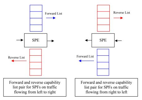
NOTE – The SPE containing the SPFs is assumed not to be an originating or terminating equipment. If it is known to be at the originating or terminating equipment, only one capability list will be sent out in each direction.
