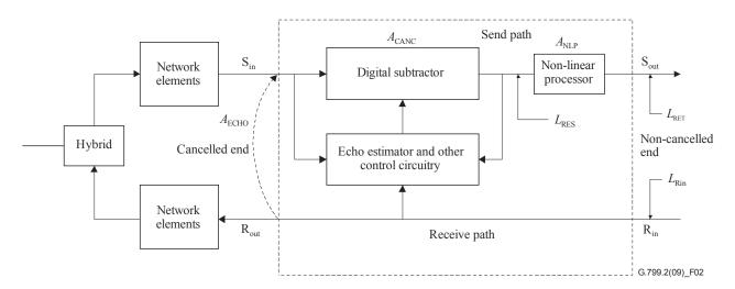
Figure 2 – Block diagram of an echo canceller [ITU-T G.168]
