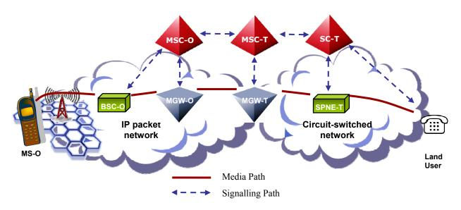
Figure I.6 – Mobile-to-land call through an IP packet network and a circuit-switched network
