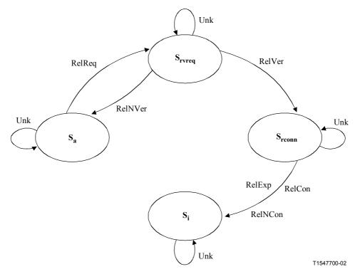
Figure 9-6/G.7713/Y.1704 – Network CallC Call Release State Diagrams
