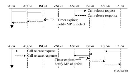
Figure 6-23/G.7713/Y.1704 – Signal flow: Release call → User Initiated Release (Network timer expires)
