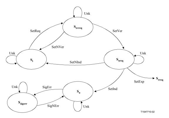
Figure 9-7/G.7713/Y.1704 – Initiating CC Connection Setup State Diagrams
