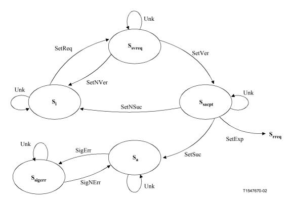
Figure 9-3/G.7713/Y.1704 – Terminating User CallC Call Setup State Diagrams
