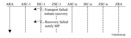
Figure 6-21/G.7713/Y.1704. Signal flow: Existing call → transport network connection defect
