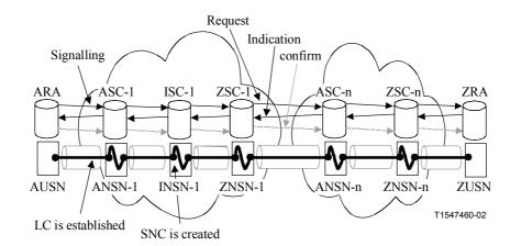
Figure 6-6/G.7713/Y.1704 – LC Establishment and SNC Creation for a Connection Setup Request
