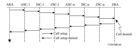
Figure 6-18/G.7713/Y.1704 – Signal flow: Setup → ZRA UNI defect (Call denied)
