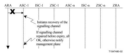
Figure 6-8/G.7713/Y.1704 – UNI Signalling defect
