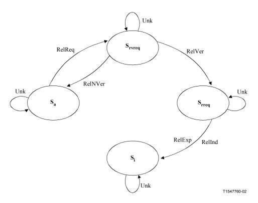
Figure 9-12/G.7713/Y.1704 – Intermediate CC Connection Release State Diagrams
