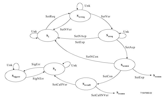
Figure 9-5/G.7713/Y.1704 – Network CallC Call Setup State Diagrams
