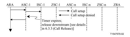
Figure 6-17/G.7713/Y.1704 – Signal flow: Setup → Intra-domain defect (Timer expires)
