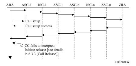
Figure 6-13/G.7713/Y.1704 – Setup → Signalling defect of the response message (ARA fails to interpret)
