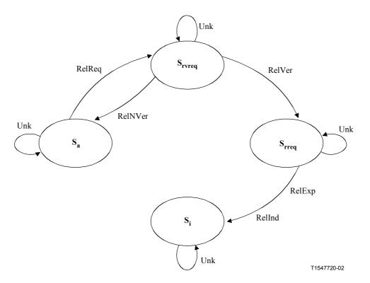
Figure 9-8/G.7713/Y.1704 – Initiating CC Connection Release State Diagrams
