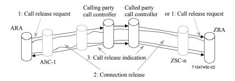
Figure 6-5/G.7713/Y.1704 – Call Release Request Processing: Logical Request Progression
