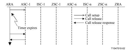
Figure 6-11/G.7713/Y.1704 – Setup → ARA UNI defect (Timer expires)
