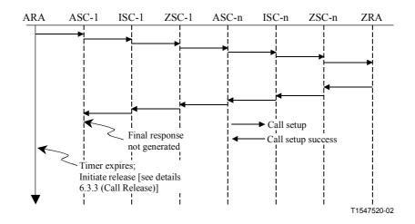
Figure 6-12/G.7713/Y.1704 – Setup → Signalling defect of the response message (final response not generated)
