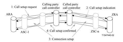
Figure 6-4/G.7713/Y.1704 – Call Setup Request Processing: Logical Request Progression
