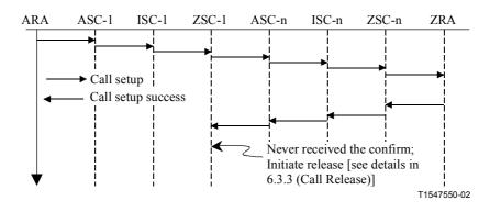
Figure 6-15/G.7713/Y.1704 – Setup → Signalling defect of the confirmation message (Confirmation message never generated)
