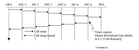
Figure 6-19/G.7713/Y.1704 – Signal flow: Setup → ZRA UNI defect (Timer expires)
