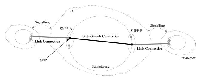
Figure 6-3/G.7713/Y.1704 – Creation of Subnetwork Connection after Link Connection Establishments
