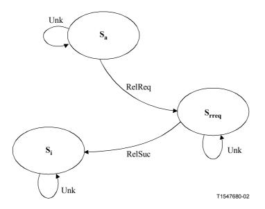
Figure 9-4/G.7713/Y.1704 – Terminating User CallC Call Release State Diagrams
