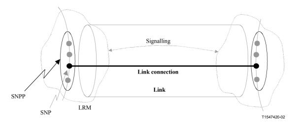
Figure 6-2G.7713/Y.1704 – Establishment of Link Connection by allocating the SNPs
