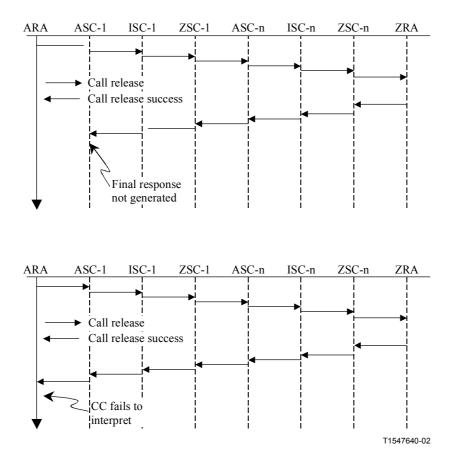
Figure 6-24/G.7713/Y.1704 – Signal Flow: Release → Signalling defect of the response message
