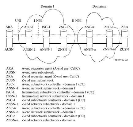
Figure 5-1/G.7713/Y.1704 – Reference diagram for distributed connection management
