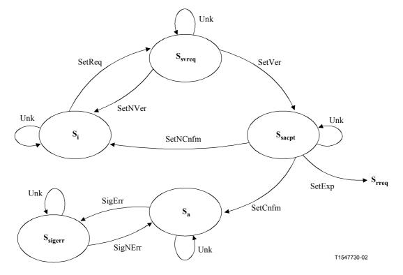
Figure 9-9/G.7713/Y.1704 – Terminating CC Connection Setup State Diagrams
