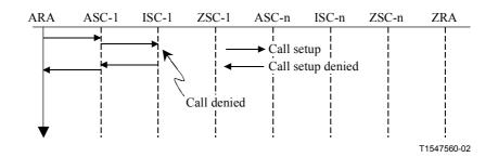
Figure 6-16/G.7713/Y.1704 – Signal flow: Setup → Intra-domain defect (Call denied)
