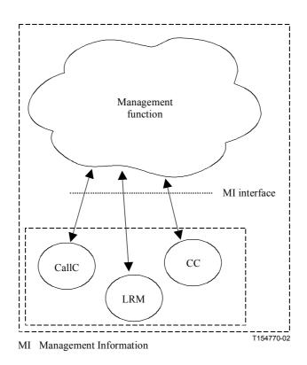
Figure 10-1/G.7713/Y.1704 – Interface between Control Plane Components and Management Plane
