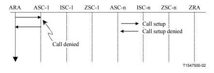
Figure 6-10/G.7713/Y.1704 – Setup → ARA UNI defect (Call denied)
