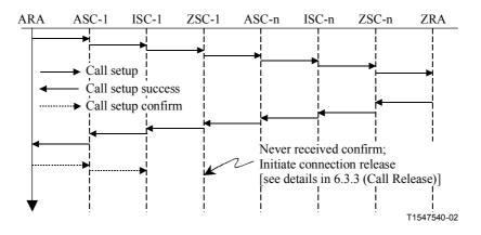
Figure 6-14/G.7713/Y.1704 – Setup → Signalling defect of the confirmation message (Confirmation message lost during transmission)
