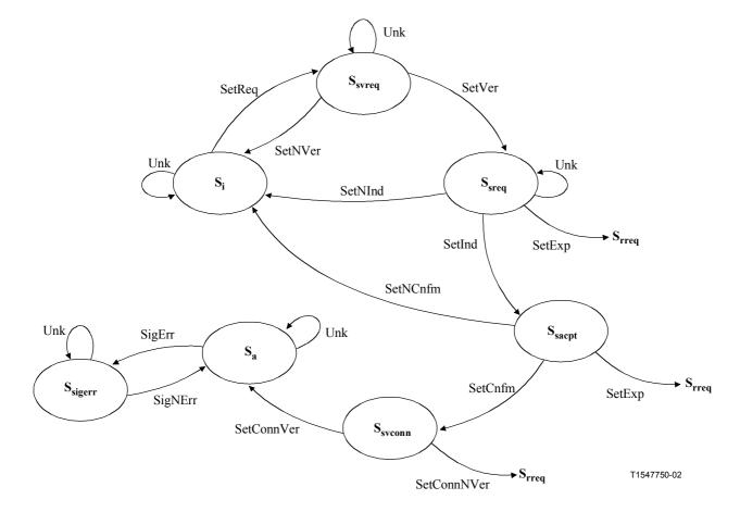
Figure 9-11/G.7713/Y.1704 – Intermediate CC Connection Setup State Diagrams
