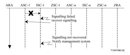
Figure 6-9/G.7713/Y.1704 – Network signalling defect
