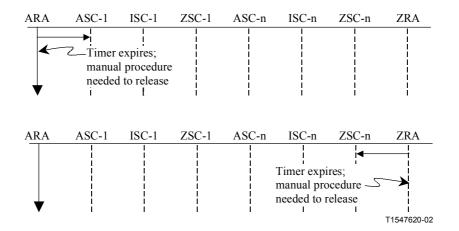
Figure 6-22/G.7713/Y.1704 – Signal flow: Release call → User Initiated Release (User Timer expires)
