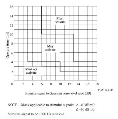
Figure I.1/G.763 – Transmit activity detection operate threshold mask
