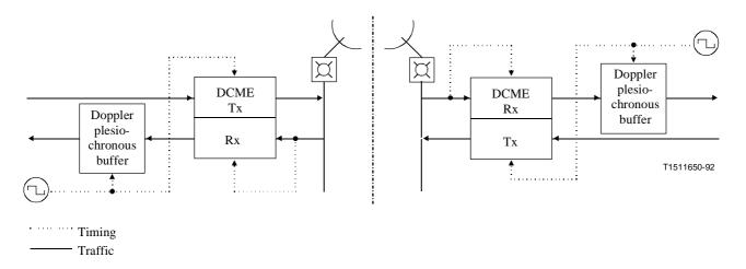
Figure I.12/G.763 – DCME synchronous (independent) operation (between two plesiochronous networks)
