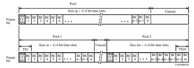
NOTE 1 – The boundary of Pool 1 and the lower boundary of Pool 2 are at the boundaries of 8-bit time slots within the G.704 bearer frame structure. Unused portions of the bearer frame will also be integers of 8-bit slots.
