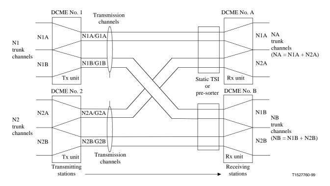
Figure 2/G.763 – Multi-clique mode (only one direction shown)
