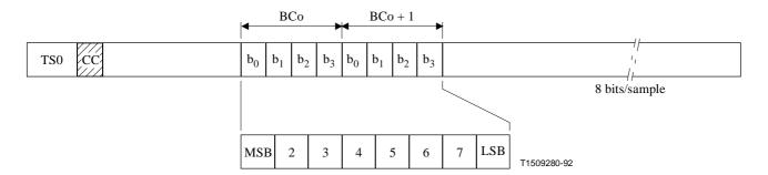
Figure 7/G.763 – 64 kbit/s (8 bits/sample) bearer channel
