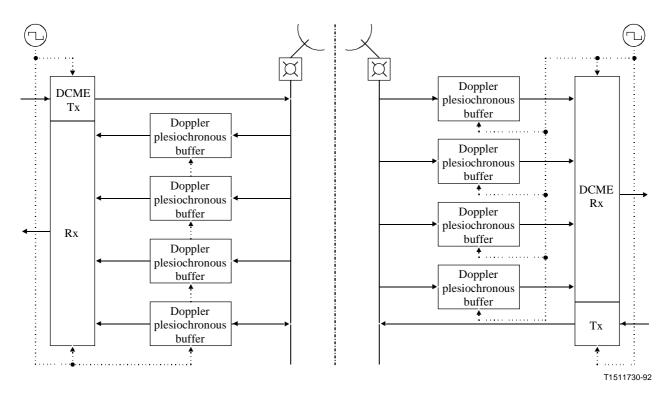
Figure I.20/G.763 – DCME buffered plesiochronous operation (between two plesiochronous networks)
