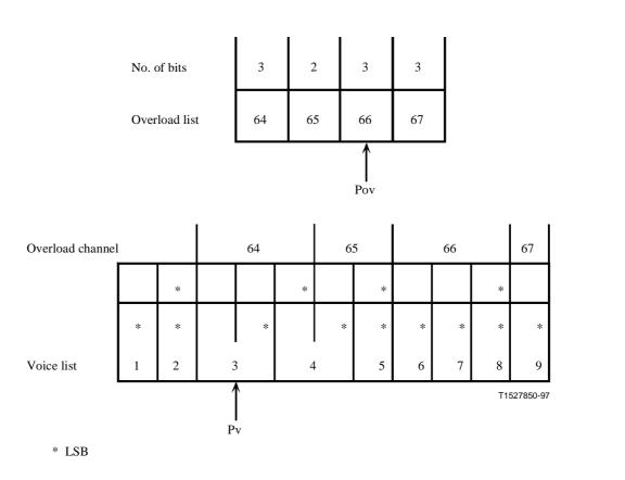
Figure 13/G.763 – Example of 3-/2-bit overload channel creation
