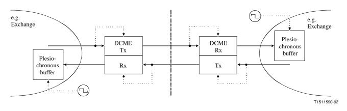
Figure I.6/G.763 – DCME synchronous (independent) operation (between two plesiochronous networks)
