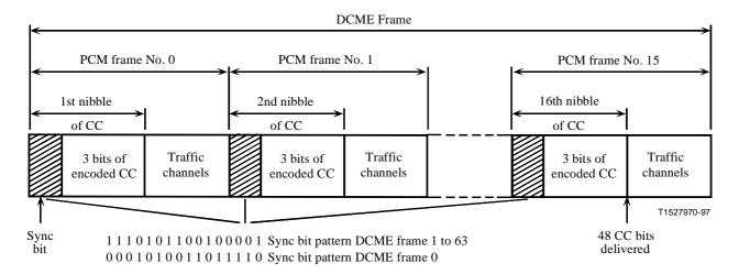
Figure 26/G.763 – CC message transmission scheme
