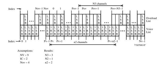
NOTE – The overload channel bits are matched with the corresponding stolen bits of the voice channels.
