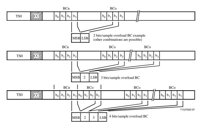
Figure 10/G.763 – An example of 32, 24 and 16 kbit/s overload bearer channels (4, 3 and 2 bits/sample)
