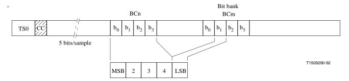
Figure 8/G.763 – 40 kbit/s (5 bits/sample) bearer channel
