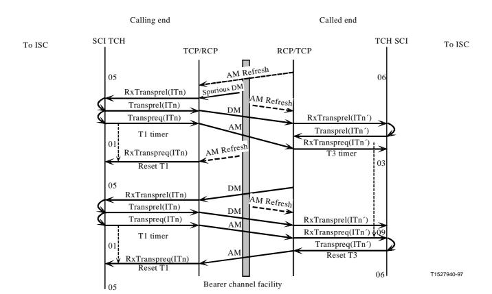
Figure 23/G.763 – Sequence chart for 64 kbit/s circuit re-establishment after a spurious disconnect into calling end
