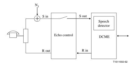
Figure I.2/G.763 – Speech detector/echo control device interactions
