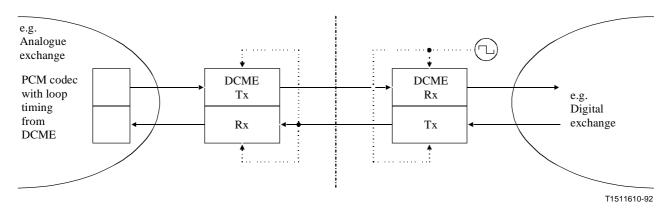
Figure I.8/G.763 – DCME synchronous loop operation (between analogue and digital networks)
