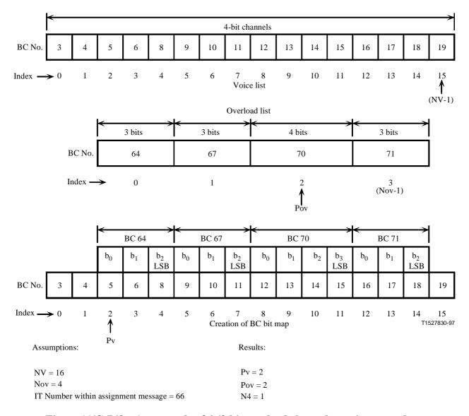
Figure 11/G.763 – An example of 4-/3-bit overload channel creation procedure
