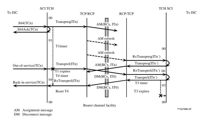
Figure 17/G.763 – Sequence chart for automatic recovery after unsuccessful (delayed) 64 kbit/s circuit establishment
