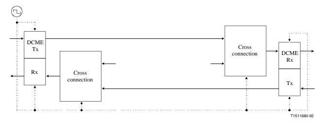
Figure I.15/G.763 – DCME synchronous operation (in a single synchronous network)
