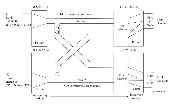
Figure 3/G.763 – Multi-destination mode (only one direction shown)
