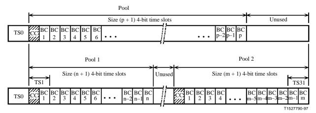
NOTE 1 – The boundary of Pool 1 and the lower boundary of Pool 2 are at the boundaries of 8-bit time slots within the G.704 bearer frame structure. Unused portions of the bearer frame will also be integers of 8-bit time slots.
