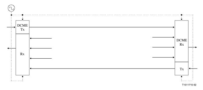
Figure I.18/G.763 – DCME synchronous operation (in a single synchronous network)
