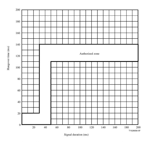
Figure 29/G.763 – Hangover time mask – ITU-T No. 5 signalling
