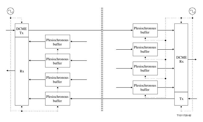
Figure I.19/G.763 – DCME buffered plesiochronous operation (between two plesiochronous networks)
