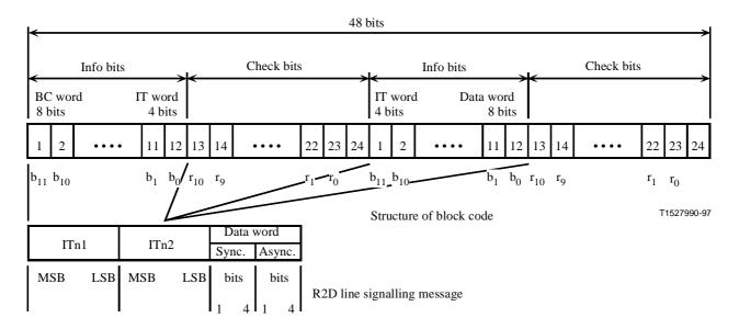
Figure 28/G.763 – R2D line signalling message format for CC
