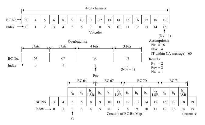
Figure A.10/G.763 – Overload channel creation process (example)
