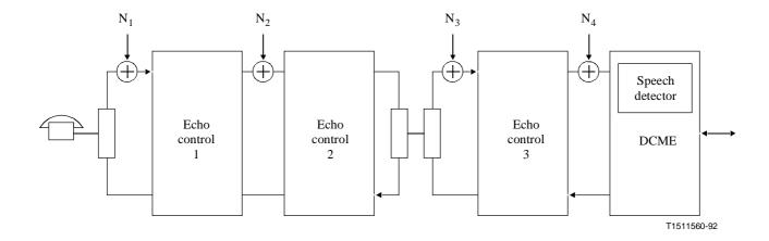
Figure I.3/G.763 – Multiple echo control device network configuration
