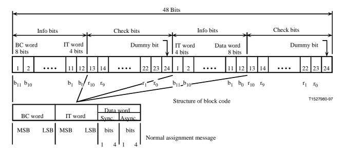
Figure 27/G.763 – DCME control channel message format
