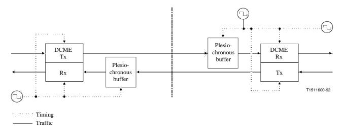
Figure I.7/G.763 – DCME buffered plesiochronous operation (between two plesiochronous networks)
