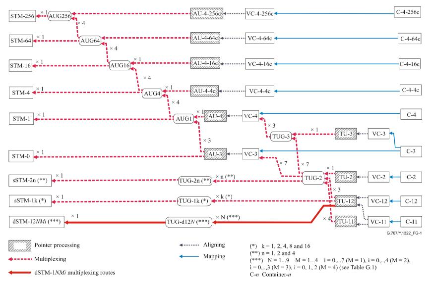
NOTE – This figure is informative and shows the additional multiplexing routes added by this Recommendation (dSTM-12NMi). It is adapted from ITU Recs G.707/Y.1322 and G.708.
