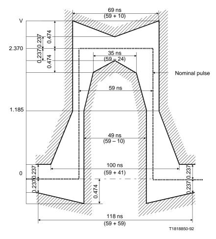
FIGURE 16/G.703 Pulse mask at the 8448-kbit/s interface
