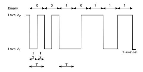
FIGURE 23/G.703 Example of CMI coded binary signal
