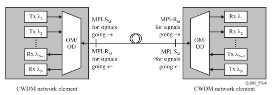
Figure 5-4/G.695 – "Black box" approach for bidirectional applications
