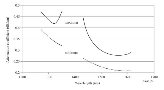
Figure I.1/G.695 – Assumed attenuation coefficient values for G.652.A&B cable
