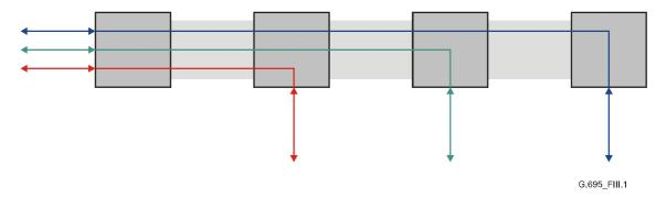
Figure III.1/G.695 – Simple example of linear black-link topology
