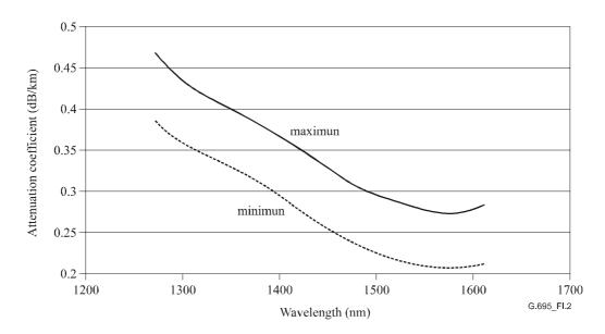
Figure I.2/G.695 – Assumed attenuation coefficient values for G.652.C&D cable
