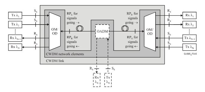
Figure 5-5/G.695 – Linear "black-link" approach for bidirectional applications
