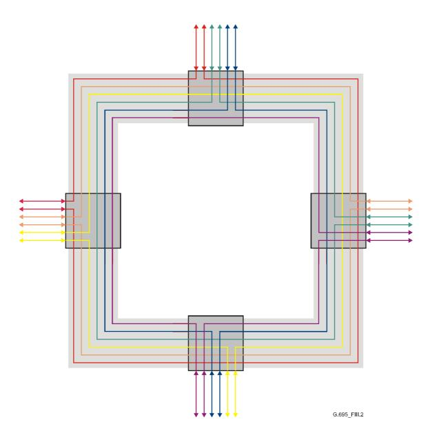
Figure III.2/G.695 – Complex example of ring black-link topology
