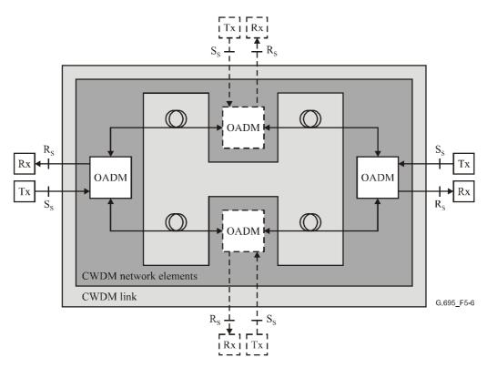
Figure 5-6/G.695 - Ring "black-link" approach for bidirectional applications
