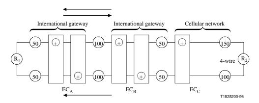
Figure I.2a/G.168 – Example of international connection originating at analogue station and terminating in a digital cellular network
