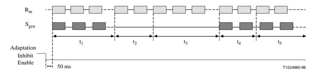
Figure 12/G.168 – Test No. 3C signal and time relationships
