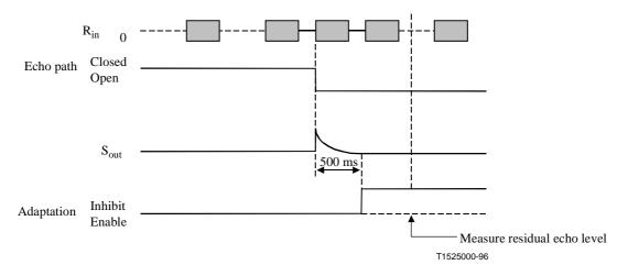
Figure 14/G.168 – Test No. 5 signal and time relationships
