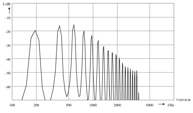
Figure C.7/G.168 – Power density spectrum of the bandlimited double talk voiced signal (analysis window: Hanning)
