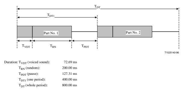
Figure C.5/G.168 – Composite Source Signals to simulate double talk (schematic)
