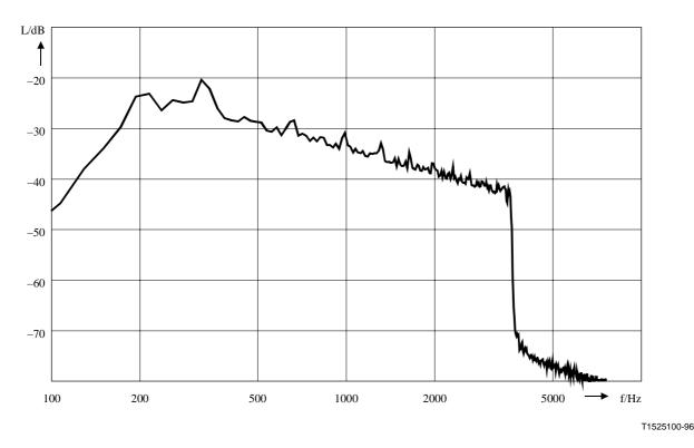
Figure C.2/G.168 – Power density spectrum of the bandlimited CSS (single talk signal, analysis window: Hanning)
