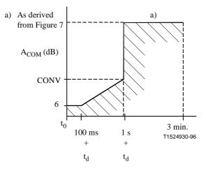
Figure 8a/G.168 – Convergence characteristics with NLP enabled
