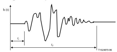
Figure 3/G.168 – Example of an impulse response of an echo path
