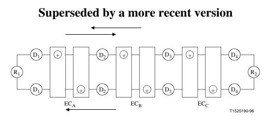
Figure I.2/G.168 – Reference connection for tandem ECs
