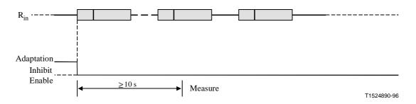
Figure 5/G.168 – Test No. 1 signal and time relationships
