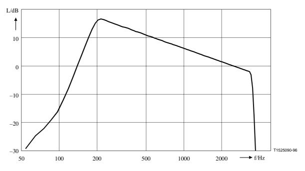
Figure C.4/G.168 – Transfer function of the filter for bandlimiting the PN-sequence
