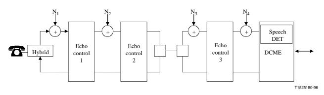
Figure I.4/G.168 – Multiple echo control devices in a DCME/PCME network configuration
