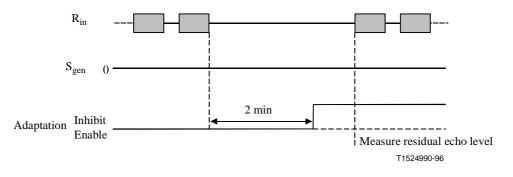
Figure 13/G.168 – Test No. 4 signal and time relationships
