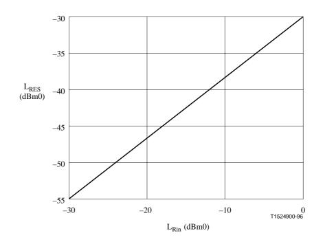
Figure 6/G.168 – Relationship between receive input level  $(L_{Rin})$  and residual echo level  $(L_{RES})$  with NLP disabled
