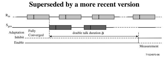
Figure 11/G.168 – Test No. 3B signal and time relationships
