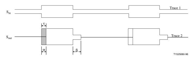
Figure B.2/G.168 – Traces for NLP operate and hangover times,  $L_{Rin}$  constant
