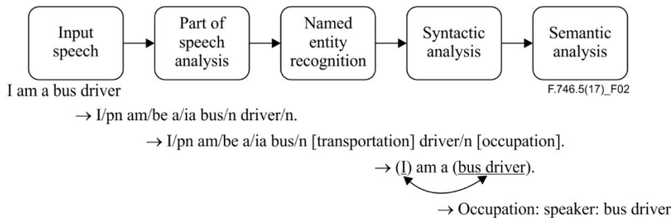
**Figure 2 – Basic NLP flows with processing modules**
