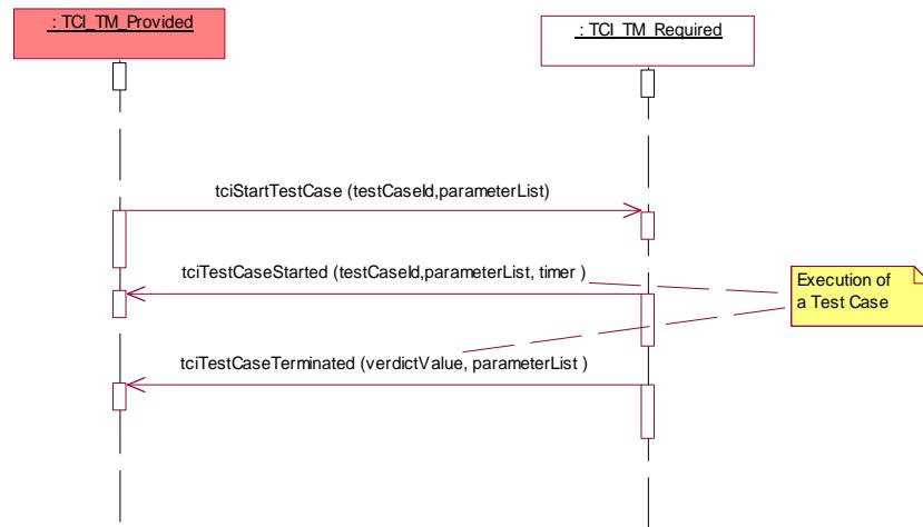
**Figure C.6 – Use scenario – direct test case execution**
