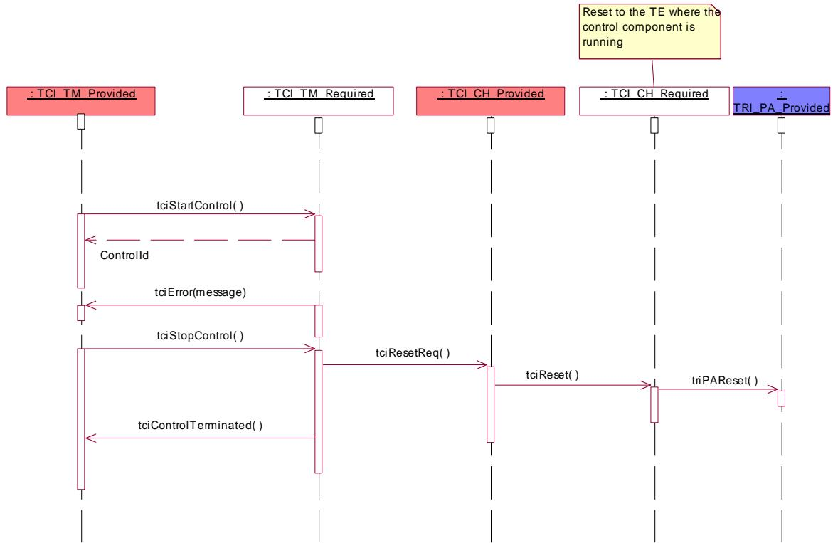
**Figure C.18 – Use scenario – termination of control after error**
