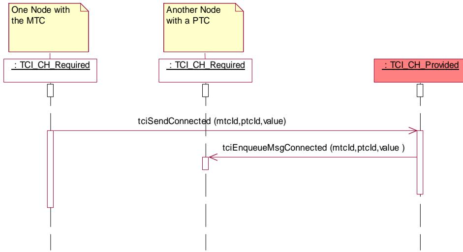
**Figure C.22 – Use scenario – internode communication between test components**
