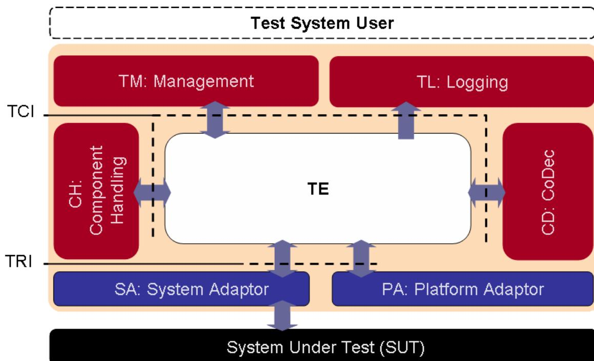
**Figure 1 – General structure of a TTCN-3 test system**
