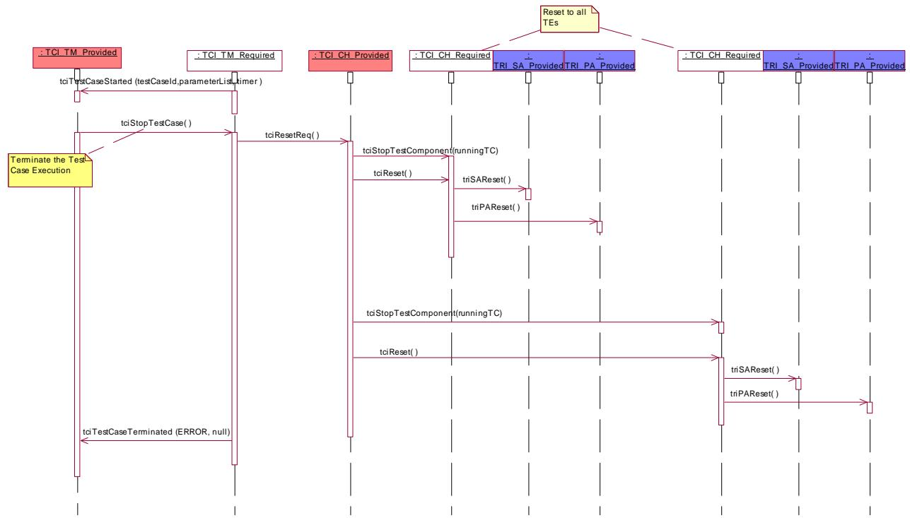
**Figure C.16 – Use scenario – stop a test case**
