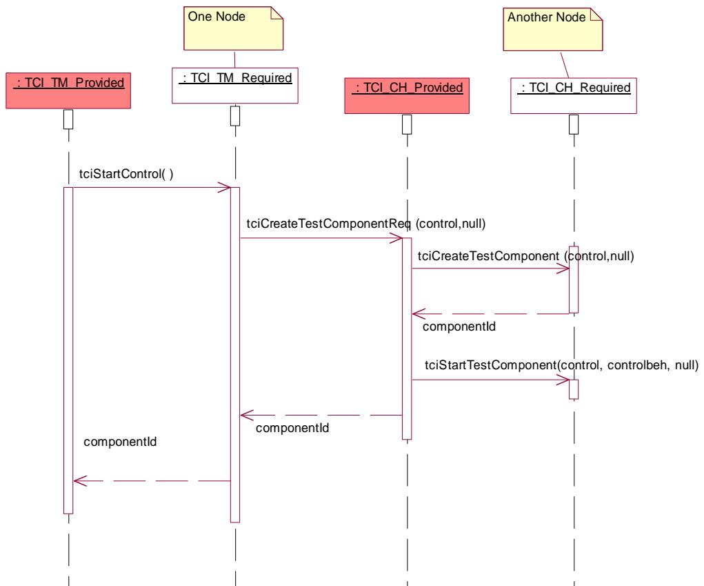
Figure C.9 – Use scenario – remote control component creation
