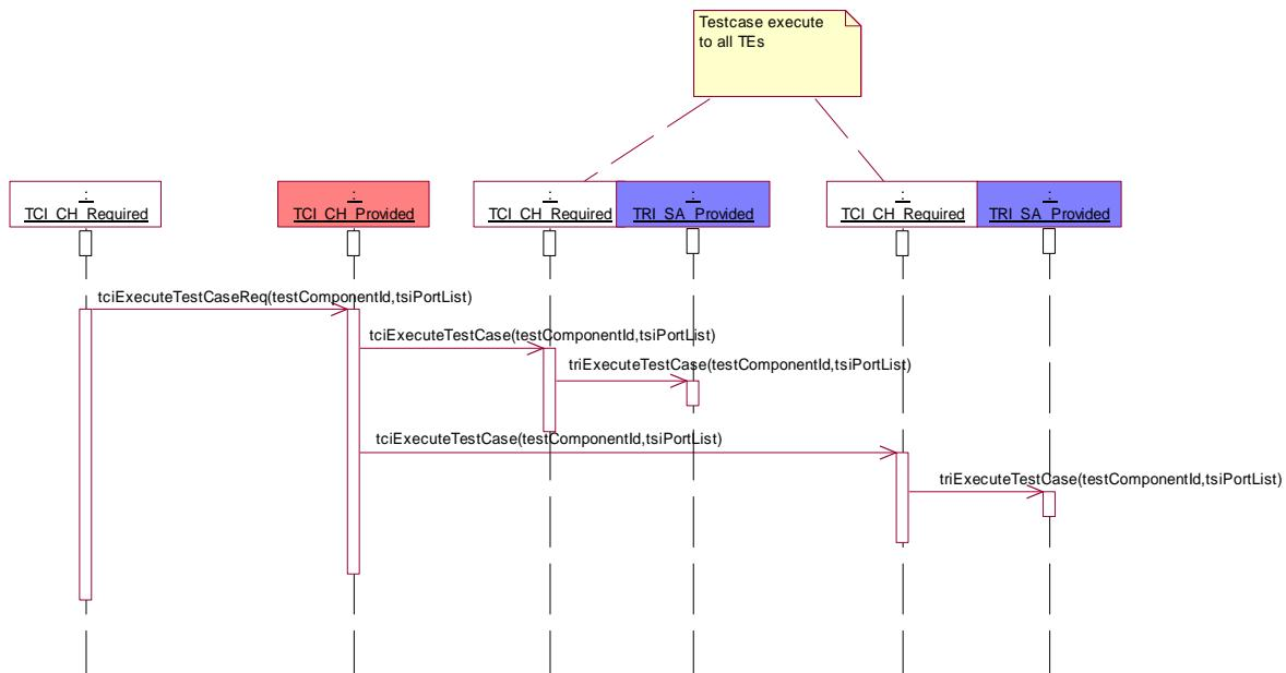
**Figure C.7 – Use scenario – execute test case to TRI**
