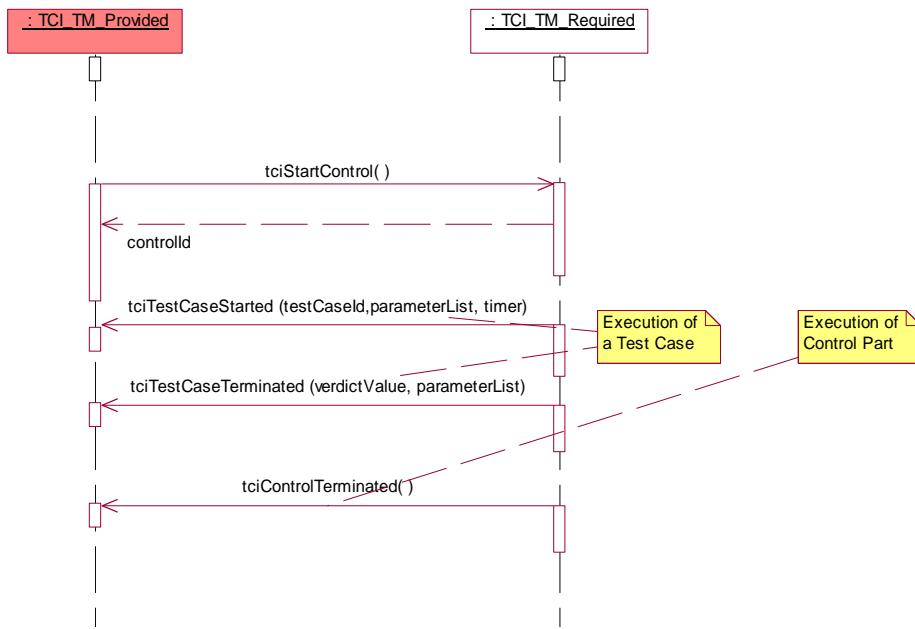
**Figure C.5 – Use scenario – test case execution within control**
