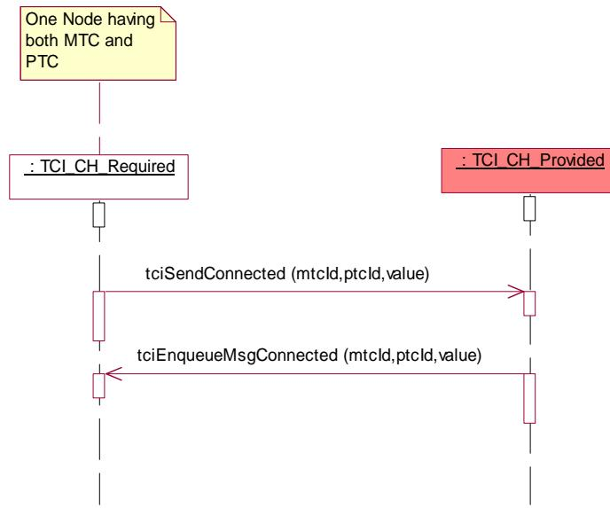
**Figure C.21 – Use scenario – local intercomponent communication**
