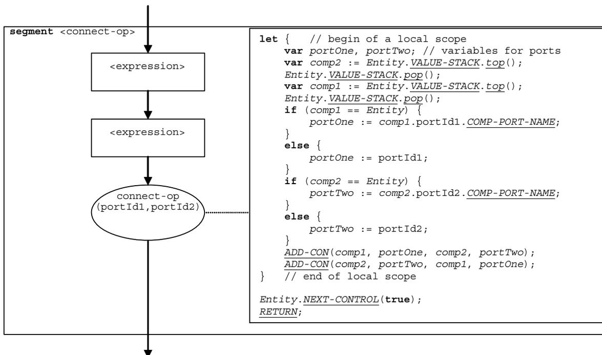
Figure 60 – Flow graph segment <connect-op>
