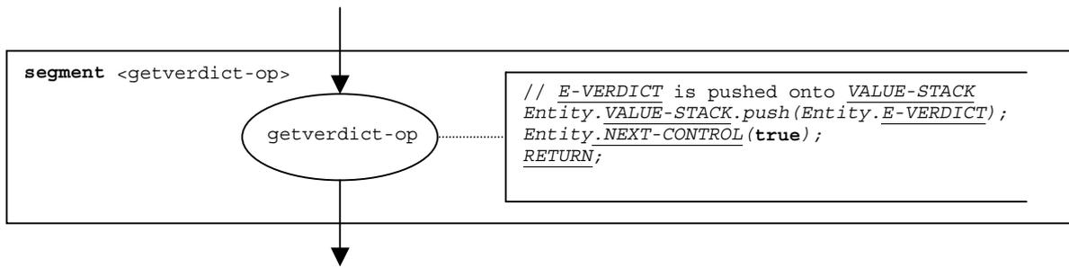
**Figure 88 – Flow graph segment `<getverdict-op>`**
