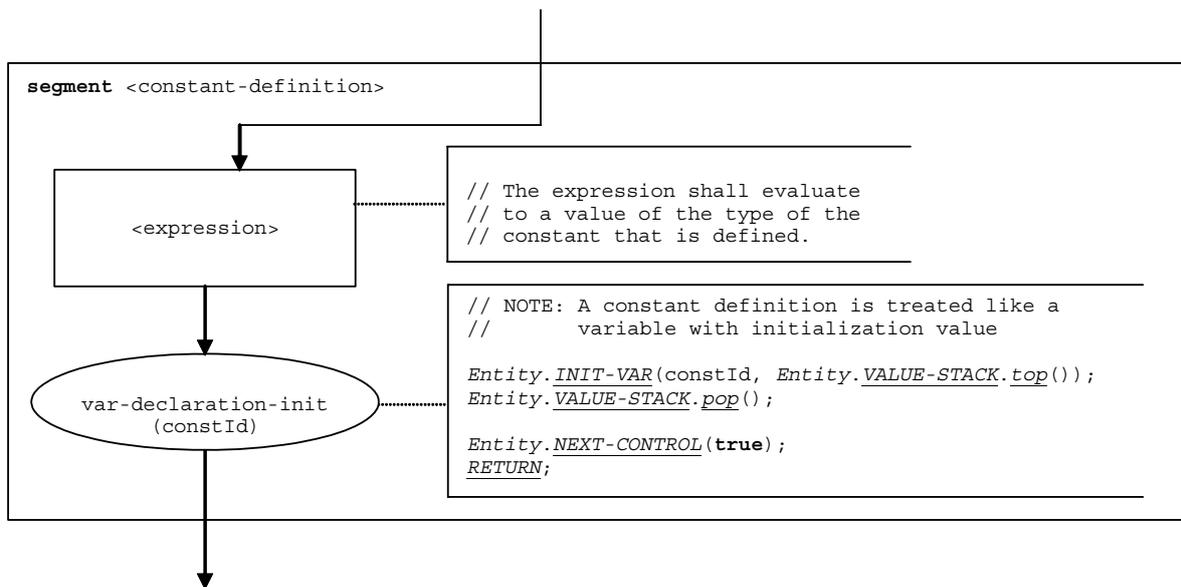
Figure 61 – Flow graph segment `<constant-definition>`
