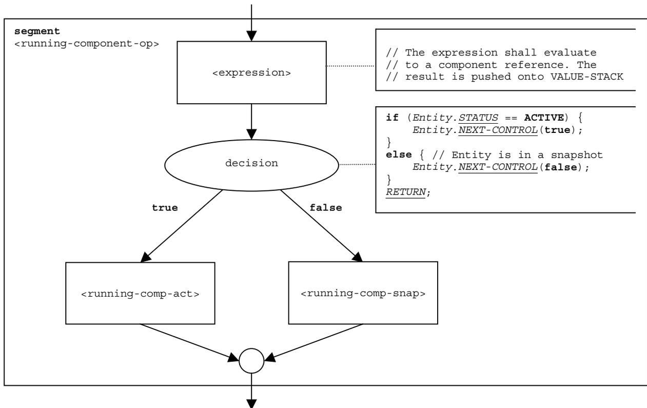
**Figure 111 – Flow graph segment `<running-component-op>`**
