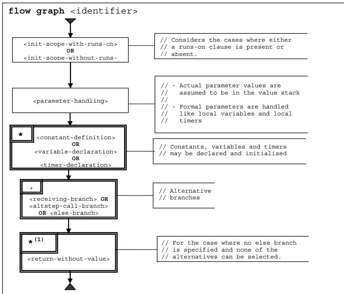
**Figure 21 – Flow graph representation of altsteps**
