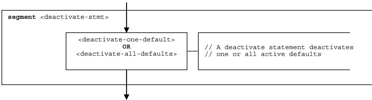
Figure 63-a – Flow graph segment `<deactivate-stmt>`
