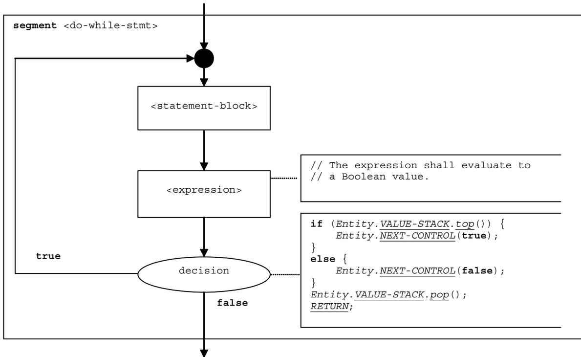
Figure 65 – Flow graph segment `<do-while-stmt>`
