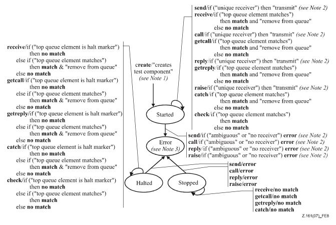
NOTE 1 – When creating a PTC, the ports of that PTC are created and started; when creating a MTC, the ports of the MTC and the ports of the TSI are created and started.
