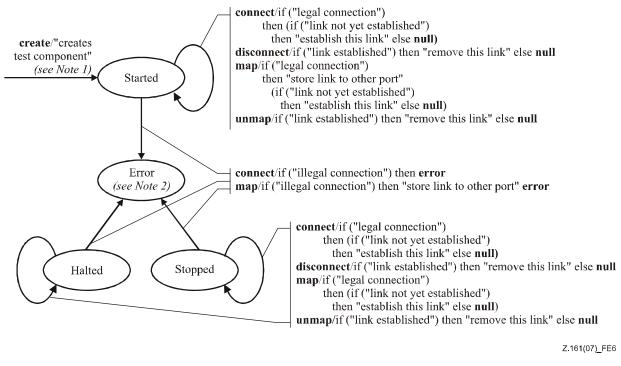
NOTE 1 – When creating a PTC, the ports of that PTC are created and started; when creating the MTC, the ports of the MTC and the ports of the TSI are created and started. NOTE 2 – Whenever a port enters its error state, the test component it belongs to enters also its error state, assigns a local error verdict, the test case terminates and the overall test case result will be an error.
