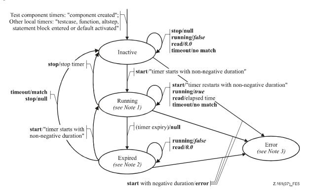
NOTE 1 – For any scope unit, all timers in that scope being in Running state constitute the running-timer list. NOTE 2 – For any scope unit, all timers in that scope being in Expired state constitute the timeout-list. NOTE 3 – Whenever a timer enters its error state, the test component it belongs to enters also its error state, assigns a local error verdict, the test case terminates and the overall test case result will be an error.
