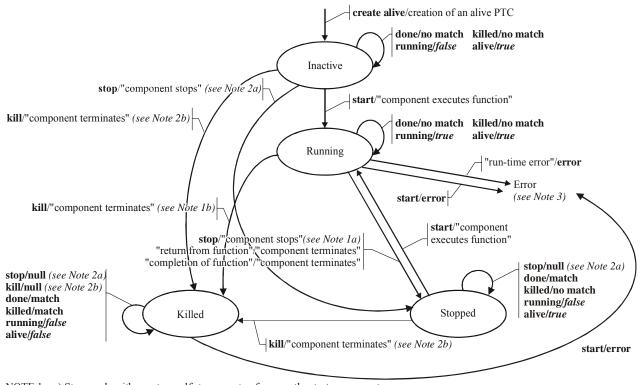
NOTE 1 – a) Stop can be either a stop, self.stop or a stop from another test component.b) Kill can be either a kill, self.kill, a kill from another test component or a kill from the test system (in error cases).
