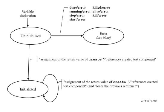
NOTE – Whenever a test component enters its error state, the error verdict is assigned to its local verdict, the test case terminates and the overall test case result will be an error.
