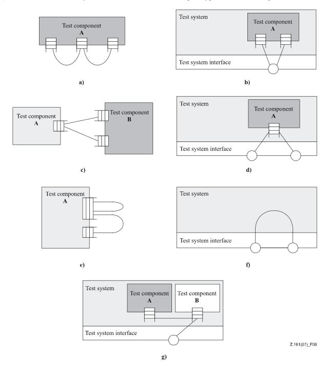
**Figure 6 – NOT allowed connections**
