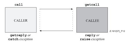
Figure 12 – Illustration of blocking procedure-based communication
