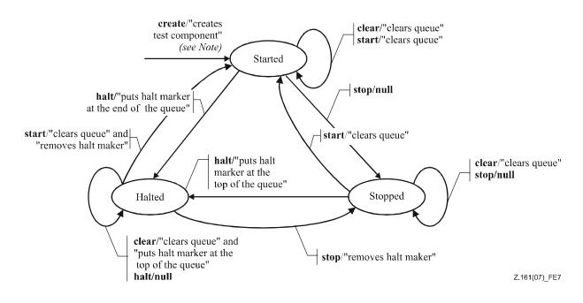
NOTE – When creating a PTC, the ports of that PTC are created and started; when creating the MTC, the ports of the MTC and the ports of the TSI are created and started.
