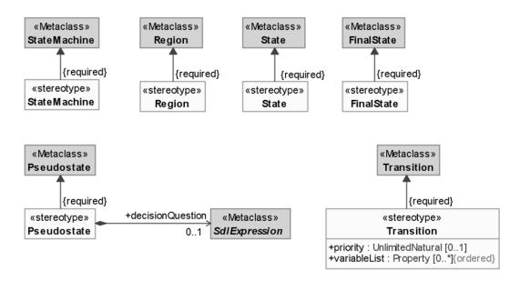
Figure 8-1 – State machine stereotypes
