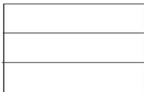
The relative positioning of the two lines dividing the <class symbol> into three compartments is allowed to be different than as shown.
