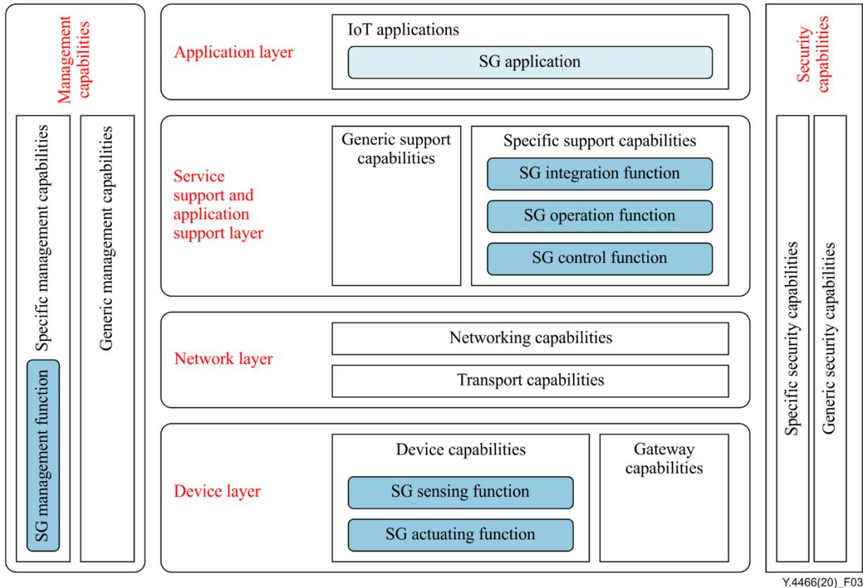
**Figure 3 – SG service reference model in accordance with the IoT reference model [ITU-T Y.4000]**
