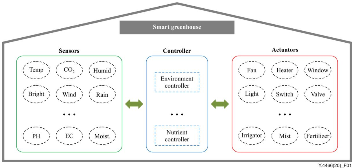
**Figure 1 – Conceptual diagram of smart greenhouse**
