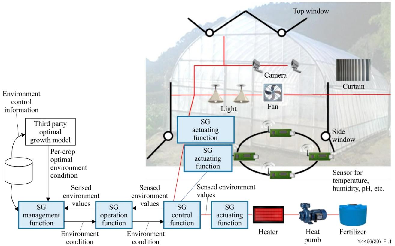
**Figure I.1 – Smart greenhouse use case**
