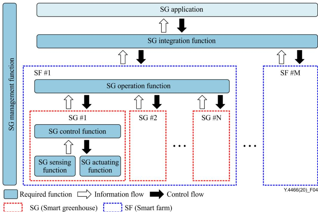
**Figure 4 – A high-level information and control flow of SG service**
