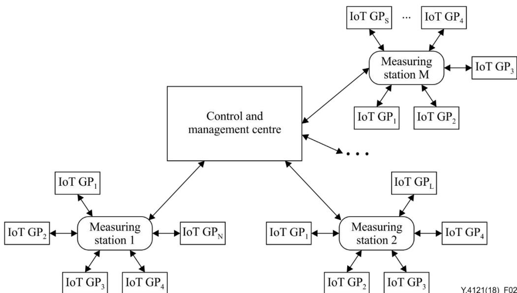
**Figure 2 – IoT GP devices placement**
