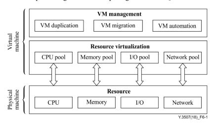
Figure 6-1 – Concept of a computing machine in [ITU-T Y.3510]
