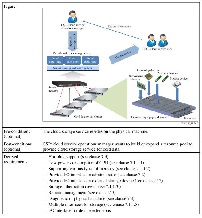
$Table \ II.4-Using \ an \ interconnect \ network \ for \ high-performance \ service-use \ case$
