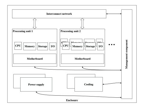
Figure 6-5 – Example of a multi-processing unit type
