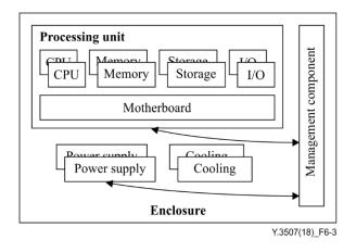
Figure 6-3 – Example of single processing unit type
